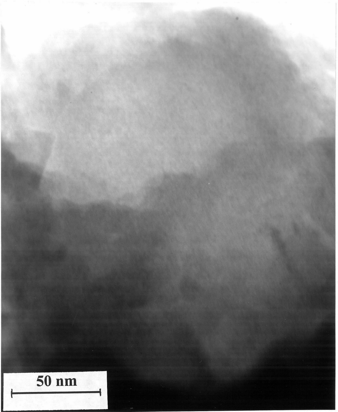
Figure 4.36 Bright field TEM Photograph of single phase amorphous phase I in \text{Al}_{60}\text{Ge}_{40} pressed to 180 kbar.
