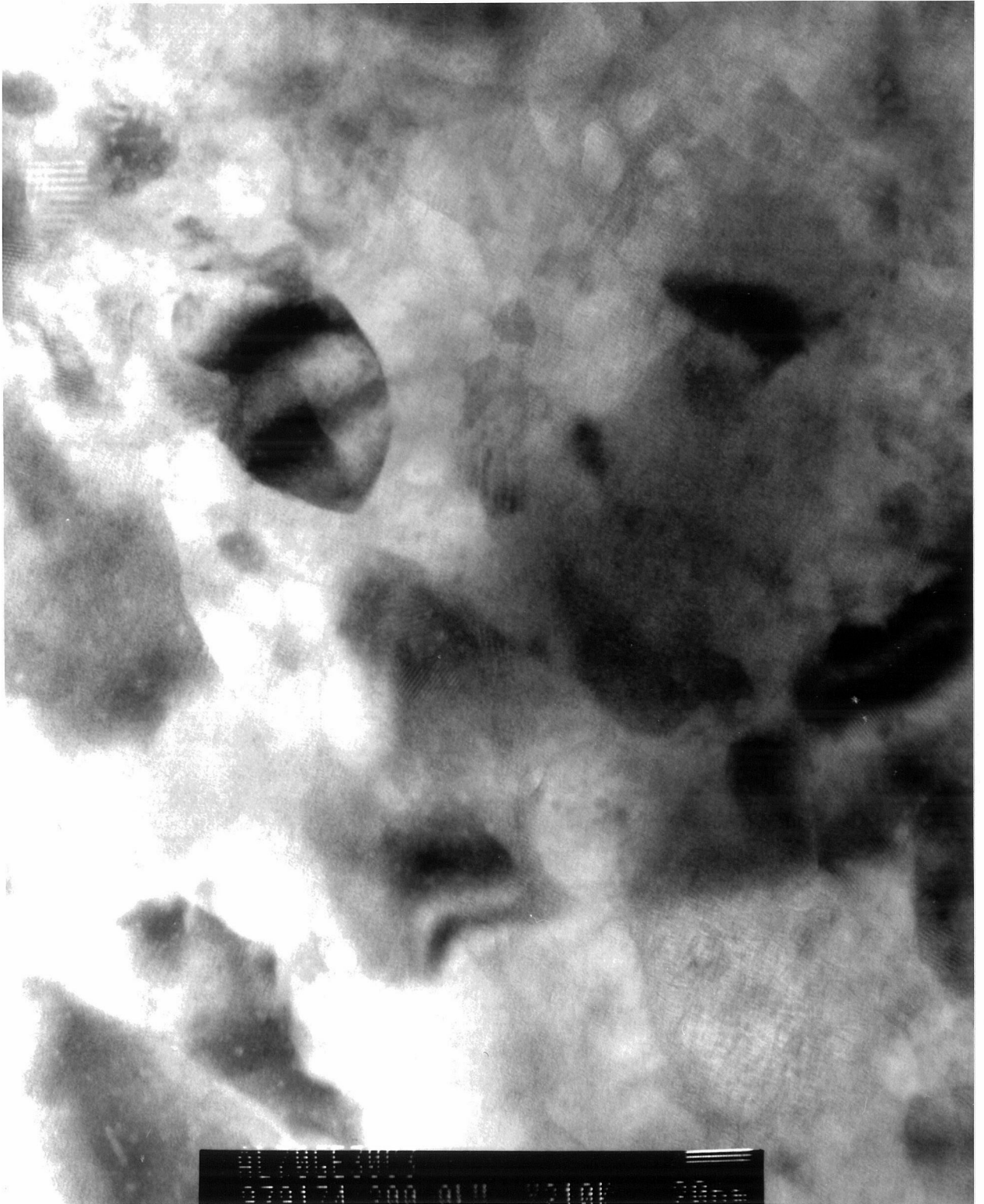
Figure 4.31 Bright field TEM Photograph of Al 70 Ge 30 pressed to 200 kbar.
