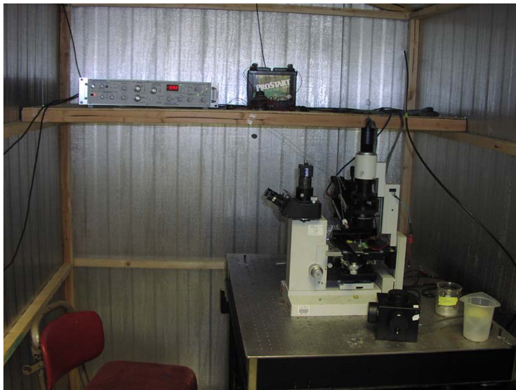
Figure 2. View of the single-channel patch clamp assembly optimized for high time resolution and low noise. Attention was paid to keep only necessary components inside the Faraday cage and to minimize the number of electrical connections entering the cage.
