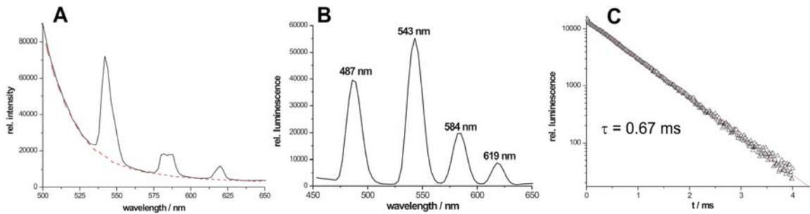
**Figure 3:** Luminescence of DOTA-Mca-labeled Ec-MscL after excitation at 336 nm. A) Emission of DOTA-Mca-labeled Ec-MscL with (solid line) and without (dashed line)  $Tb^{3+}$  after CW excitation and detection; B)  $Tb^{3+}$  luminescence, after pulsed excitation with a 10  $\mu$ s pulse and gated detection (50  $\mu$ s delay); C) Semi-logarithmic plot of  $Tb^{3+}$ -luminescence decay.
