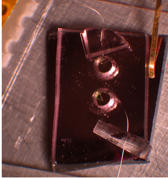
Figure 5.7: Photograph of the measurement setup showing PDMS reservoirs and platinum wire electrodes.
