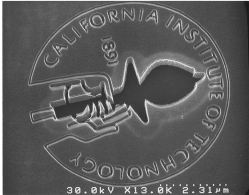
Figure 4.5: Oblique view of the Caltech logo machined in the top layer of an SOI wafer using the same PMMA layer as the electron beam resist and the etch mask during XeF_2 CAIBE processing.
