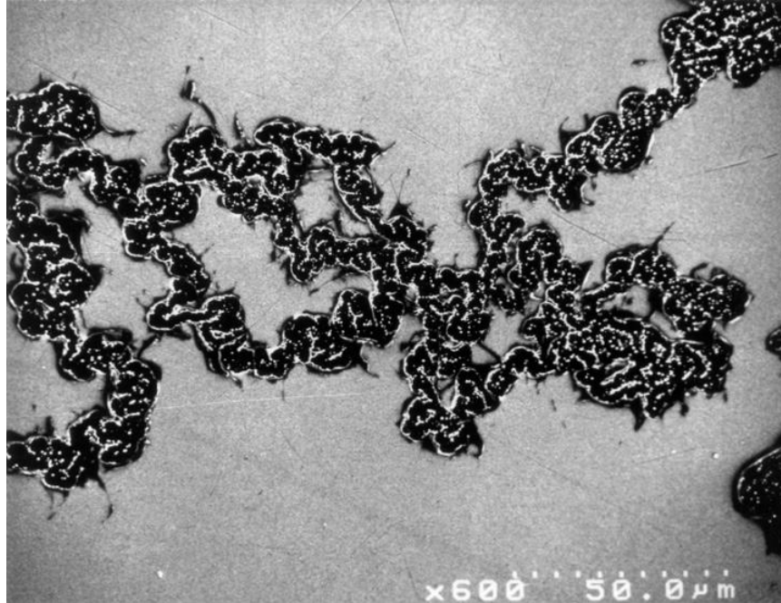
Figure 4.2: Neutralizing arc damage on a fused silica wafer.
