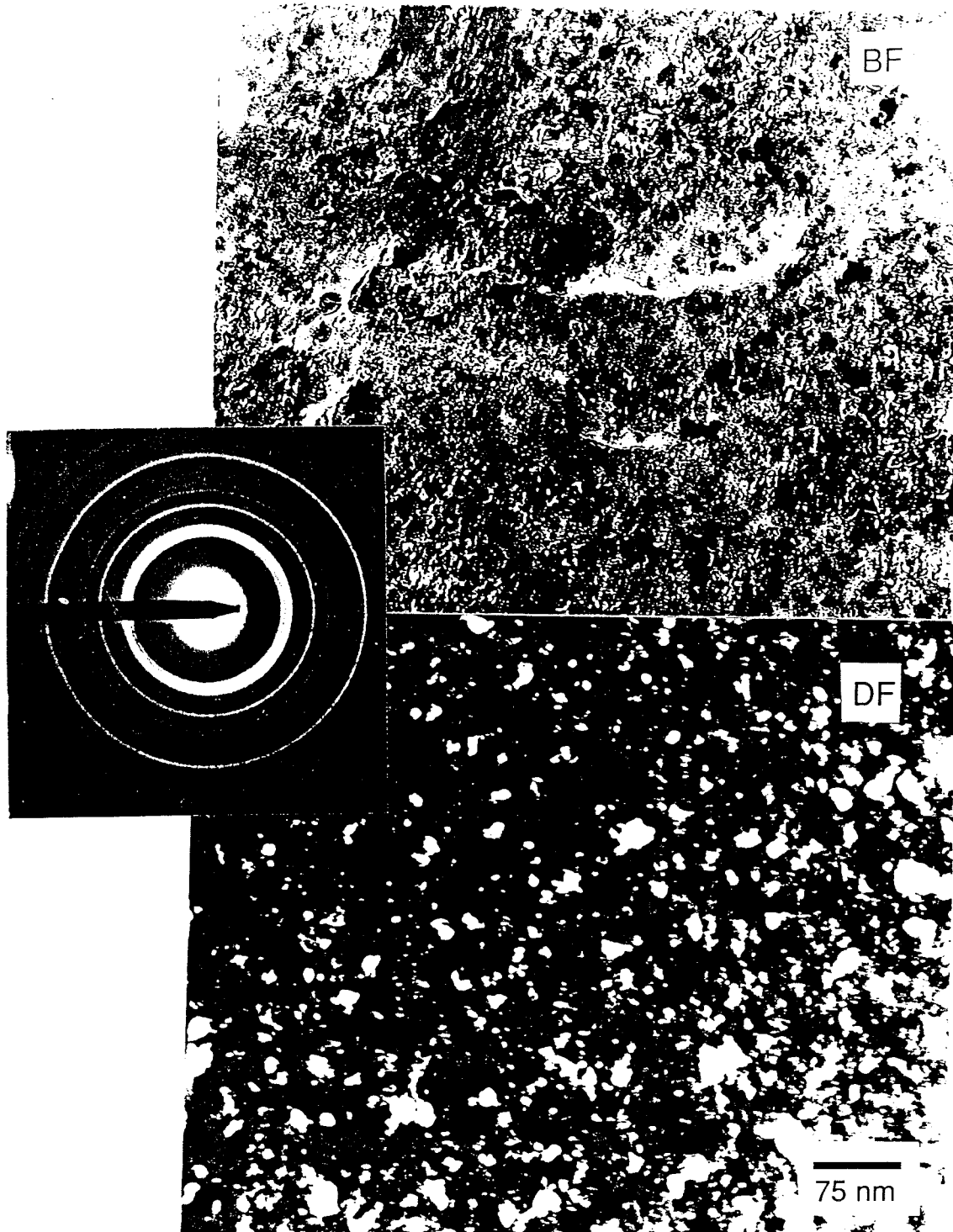
Figure 3.12. Bright field (BF) and dark field (DF) image pair and diffraction pattern from as-prepared thin film of \text{TiO}_2 .
