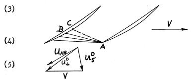
allow for fluctuations in back pressure the design pressure at (5) should be lower than the design pressure along the characteristic A-B, so that normally there would be an expansion region following A-B. A more detailed investigation might show whether or not an oblique shock along A-C would occur and be stable if the pressure at (5) exceeded the design pressure at A-B.
