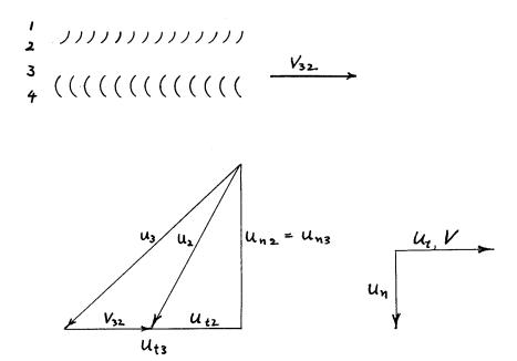
The schematic sketch above of the arrangement with the corresponding velocity diagram shows the assumed positive directions of  $u_t$ , V, and  $u_n$ . We can write down the relation between the velocities immediately:
