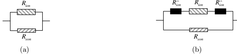
Figure 2.15: A.C. equivalent circuits representing that of Figure 2.13(a) in (a) the high-frequency limit in which all capacitors are shorted, and (b) the low-frequency limit in which all capacitors are open.
