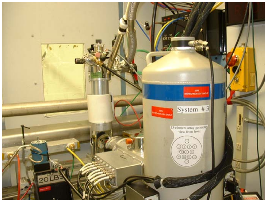
Fig. 4-2 (b) Photo of the EXAFS experimental setup chamber
