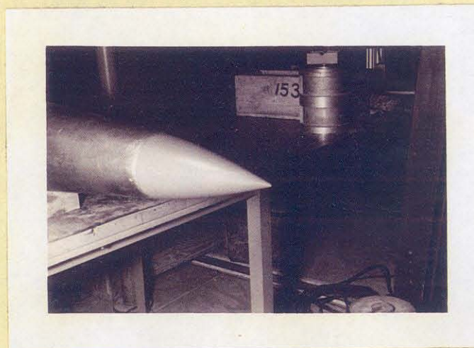
Fig. 15 Tail Cone used for Power-off Tests
