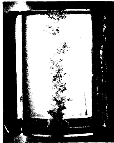
Fig. 18. Freon cavity. T=96.0^{\circ}\text{F} , v=17.52 ft/sec, l=13/16 in.
