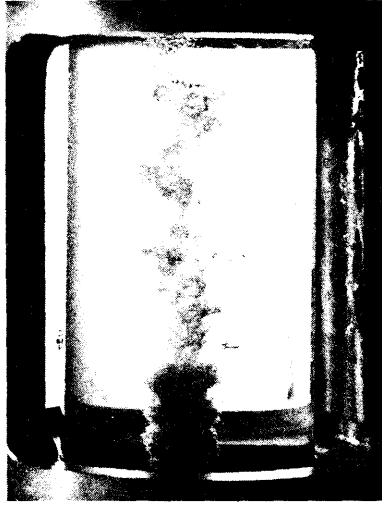
Fig. 23. Freon cavity. T=150.0^{\circ}\text{F} , v=17.39 ft/sec, l=13/16 in.
