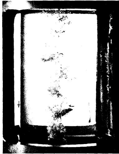
Fig. 22. Freon cavity. T=135.0^{\circ}\text{F} , v=13.82 ft/sec, l=13/16 in.
