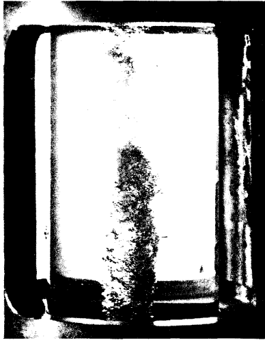
Fig. 26. Freon cavity. T=122.0^{\circ}\text{F} , v=14.70 ft/sec, l=13/8 in.
