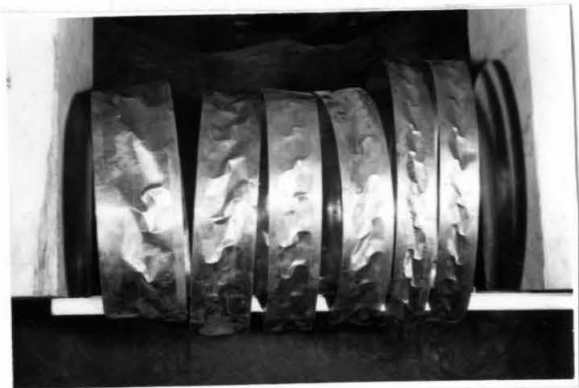
Fig. 6 Failure with Torsion
