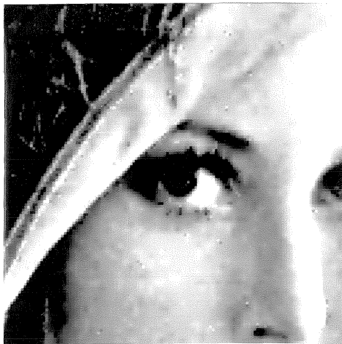
Figure 3.8.14 Quantized image of 3.8.13 by the proposed scheme with 1.07bpp and PSNR of 32.64dB and 35.32dB compared to noisy and clean original images, respectively.
