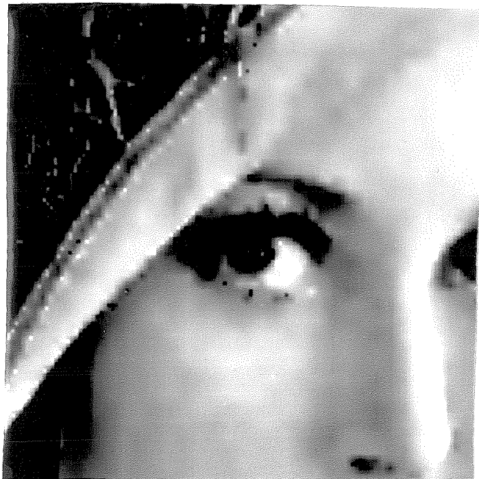
Figure 3.8.11(a) Quantized Lenna image by the proposed scheme with 0.36bpp and PSNR 32.75dB.
