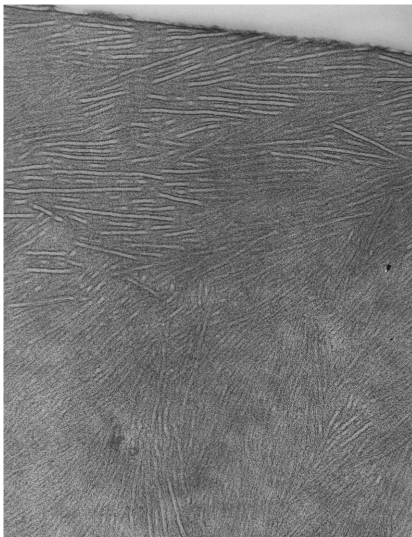
Figure 3.17: TEM of B0 crystallized quiescently at 137 °C on the surface of a quartz window. The lamellae are not ordered like those that occurred following flow. No transcrystalline layer emanates from the glass, indicating that it does not act as a nucleating surface; instead, the lamellae are part of large spherulites centered away from the glass interface. The scale bar is 100 nm.
