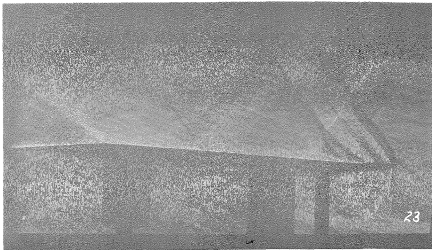
Turbulent boundary layer over probe produced by small wire at leading edge.
