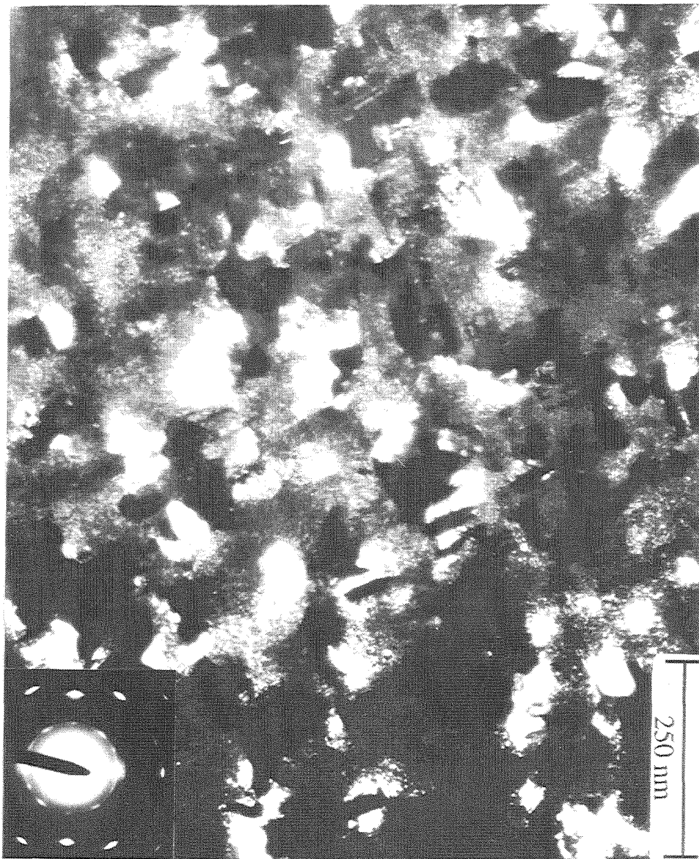
Figure 5.6: Plan view dark field transmission electron micrographs of epitaxial \text{Ni}_{80}\text{Fe}_{20} film on \text{Cu}/\text{Si}(001) , viewed along [211] zone axis with \vec{g} = [\bar{1}11] .
