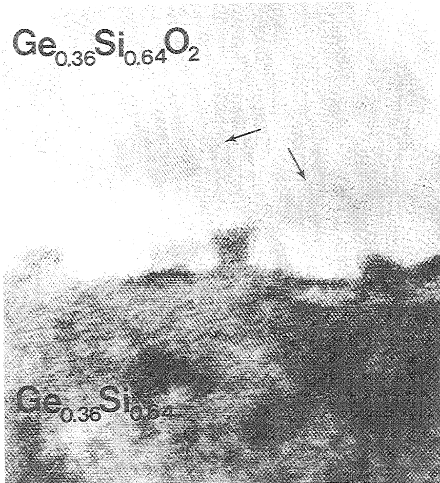
Fig. 5.2 High resolution cross-sectional transmission electron micrograph of a GeSi/GeSiO 2 interfacial region after aging for 5 months in air at room temperature. Crystalline precipitates with a lattice constant similar to that of the underlying GeSi layer are observed near the interface as the arrows indicate.
