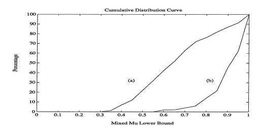
Figure 7.1: Comparison of (a) standard power iteration, and (b) adaptive power iteration on nogap matrices, with the uncertainty structure consisting of 4 real scalars, 2 complex scalars, and a  $2 \times 2$  full complex block
