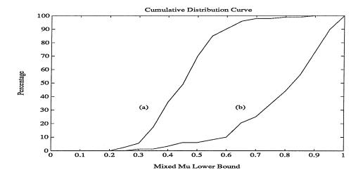
Figure 7.2: Comparison of (a) standard power iteration, and (b) adaptive power iteration on nogap matrices, with the uncertainty structure consisting of 8 real scalars, 2 complex scalars, and a  $2 \times 2$  full complex block
