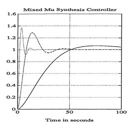
Figure 11.14: Closed loop step responses for  $k_p = 0.1,1,10$  for the Bode and mixed  $\mu$  synthesis controllers (C. D. player problem)
