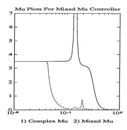
Figure 11.10: Nyquist and  $\mu$  plots for mixed  $\mu$  synthesis controller (gain margin problem)
