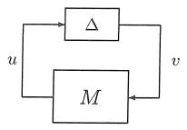
Figure 2.1: Robust stability  $\mu$  analysis framework
