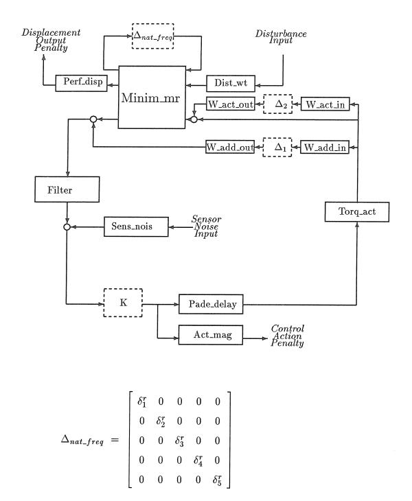
Figure 11.3: Interconnection for robust performance mixed  $\mu$  analysis of the Langley Minimast structure
