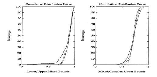
Figure 6.3: Ratios of mixed  $\mu$  lower/upper bounds, and mixed- $\mu$ /complex- $\mu$  (upper) bounds, for a sample of sysrand matrices of sizes 10 (solid), 20 (dashed), 30 (dotted), and 50 (dashdot)
