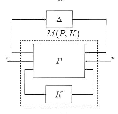
Figure 10.1: Feedback interconnection for  $\mu$  synthesis
