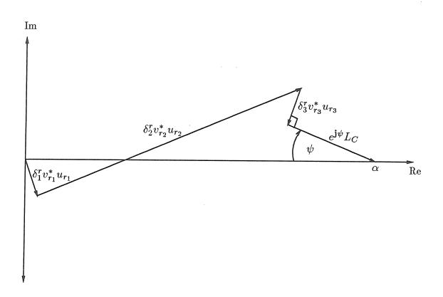
Figure 8.1: Graphical solution of the rank one mixed  $\mu$  problem
