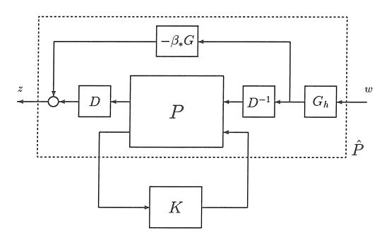
Figure 10.3: The "K" iteration of the "D,G-K iteration" procedure
