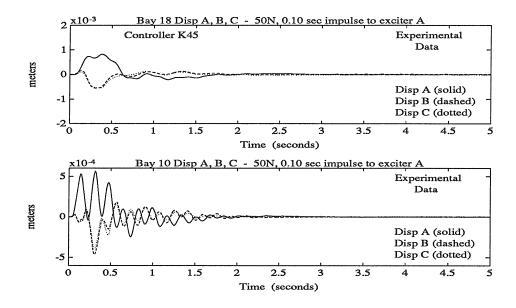
Figure 11.5: Experimental closed loop response of Langley Minimast structure to impulse input disturbance
