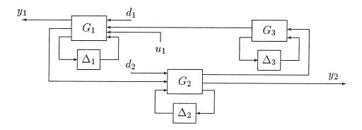
Figure 2.4: Example interconnection of LFT's
