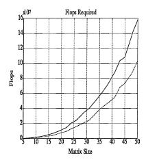
Figure 6.1: Typical computation requirements versus matrix size for mixed  $\mu$  problem (solid) and complex  $\mu$  problem (dashed)
