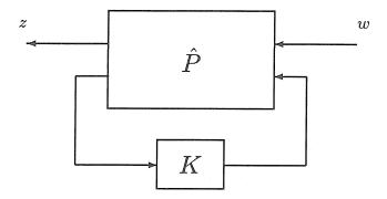
Figure 10.2: Standard framework for  $\mathcal{H}_{\infty}$  optimal control
