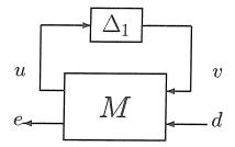
Figure 2.2: Robust performance  $\mu$  analysis framework
