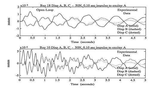
Figure 11.2: Experimental open loop response of Langley Minimast structure to impulse input disturbance
