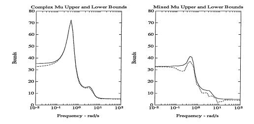
Figure 6.4: Complex  $\mu$  and mixed  $\mu$  upper & lower bounds versus frequency for a random system
