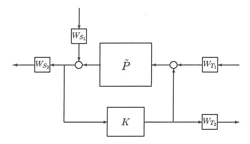
Figure 11.6: Interconnection for mixed  $\mu$  synthesis examples
