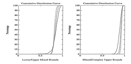
Figure 6.2: Ratios of mixed  $\mu$  lower/upper bounds, and mixed  $\mu$ /complex  $\mu$  (upper) bounds, for a sample of *crand* matrices of sizes 10 (solid), 20 (dashed), 30 (dotted), and 50 (dashdot)
