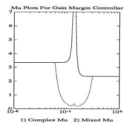
Figure 11.8: Nyquist and  $\mu$  plots for optimal gain margin controller (gain margin problem)
