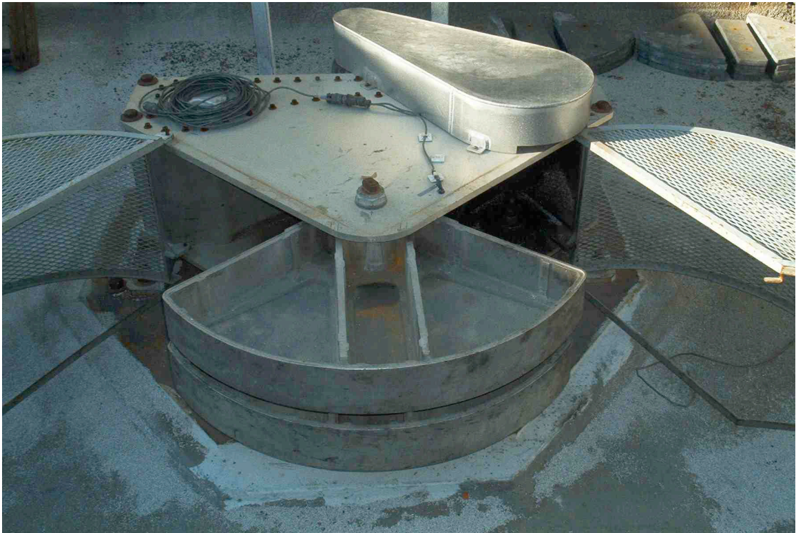
Figure B.4: Kinometrics VG-1 Synchronized Vibration Generator (Shaker). The counter-rotating buckets, shown empty, can be loaded with different configurations of lead weights. The shaker is located on the roof of Millikan Library, as shown in Figure B.2.
