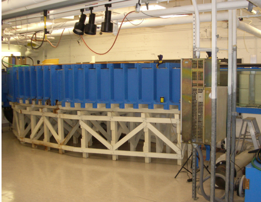
Figure 3.1: General layout of the Noah Water Tunnel. The settling chamber is visible on the left with the contraction in the middle and the test section on the far right. Visible in front of the test section is the water tunnel motor controller.
