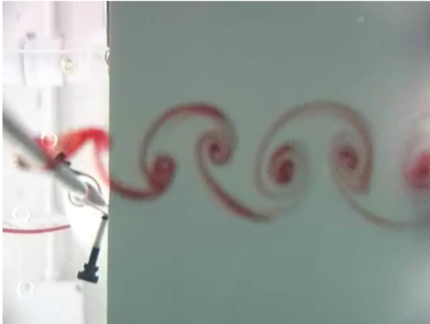
Figure 5.16: Flow visualization showing a 2S wake structure for an oscillating cylinder at its maximum amplitude, A_{\text{Max}}^* \approx 0.35 , for \text{Re} = 200
