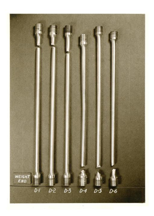
Fig. 13 D Specimens After Fracture
