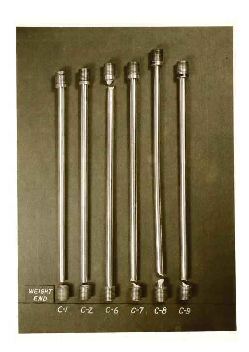
Fig. 10 C Specimens After Fracture
