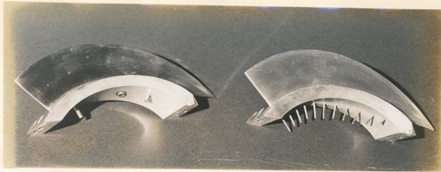
Figure 7c - Brass master blade on left and reproduction on right.
