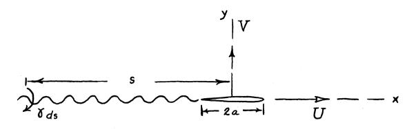
The airfoil is defined by the coordinate  $x = a \cdot cos \theta$ Note: The interference of vortex wake is investigated with the circulation being adjusted to give finite velocity at the trailing edge of the airfoil. Circulation
