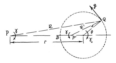
Tangential velocity  $q_2$  caused by vortex wake at the point  $oldsymbol{Q}$  of the circumference
