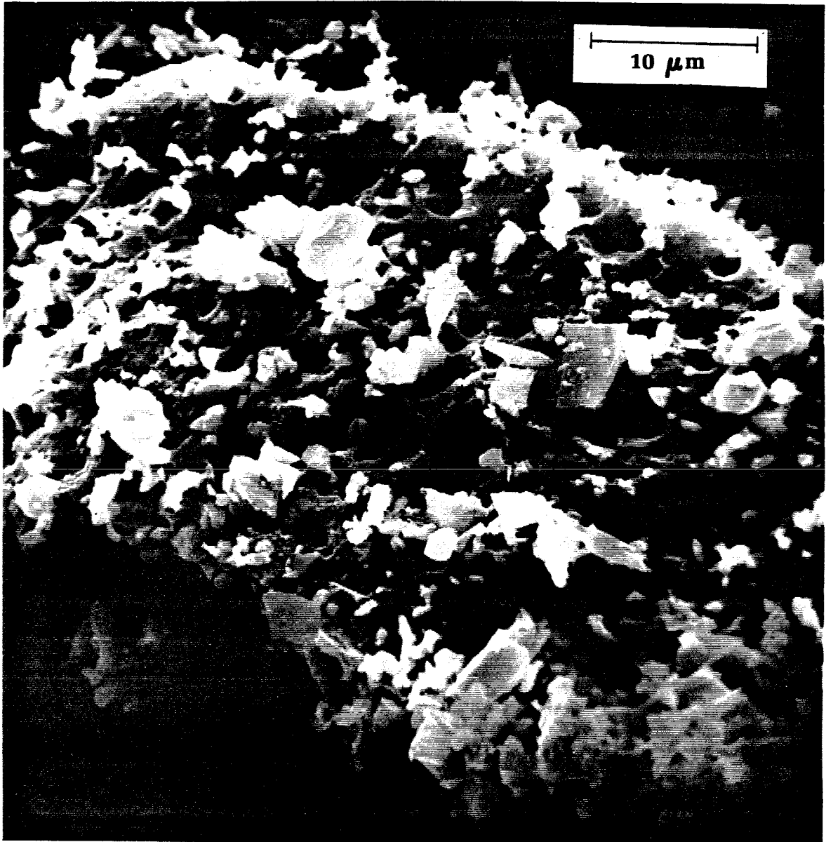
Figure 9.4a Partially burned porous carbon (magnified 1700 times).
