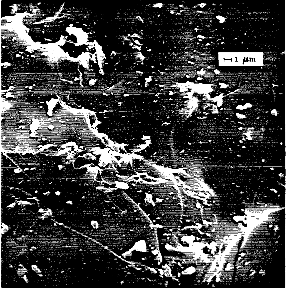
Figure 9.1 a Non-porous carbon devolatilized in N 2 at 1575 K (magnified 2000 times).
