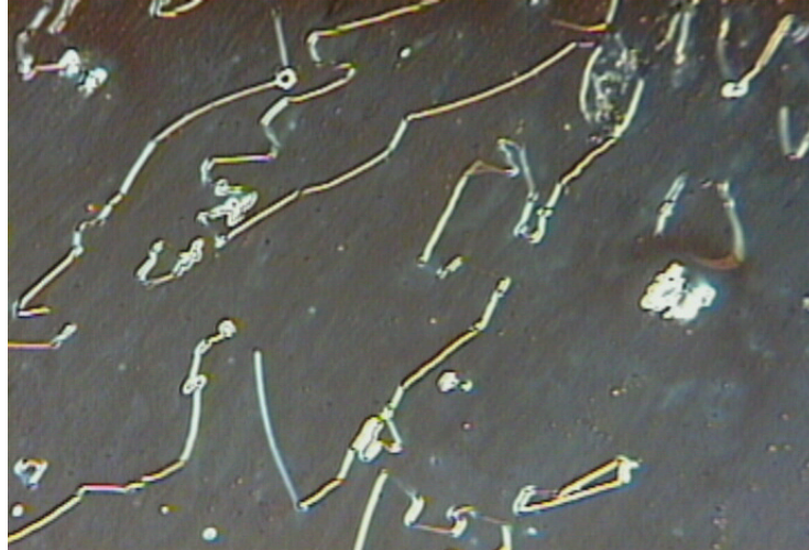
Figure 3.11: Polarization interference microscopy image of LC domains. The bright lines are the domain walls formed by LC aligning differently in response to an applied electric field as in figure 3.10
