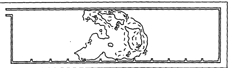
Figure 4.26(a) through (f): Contour plots of chemiluminescence images for chamber with expansion ratio of 12.0 at various phases in cycle.
