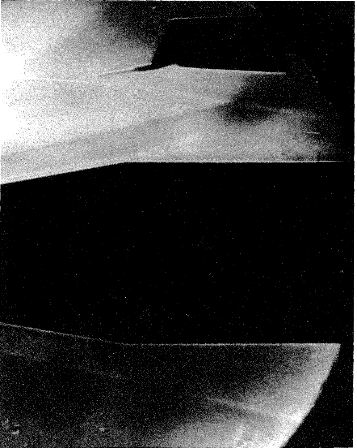
Figure 21. Schlieren Photograph of Flow Around Sharp Cone-Cylinder Juncture for Re_{R_\infty} = .08445 \times 10^6 and M_\infty = 7.87
