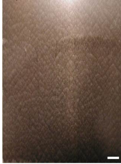
Figure 2.7: An image of a soot foil for an ethylene-oxygen mixture of equivalence ratio 2.5. The initial temperature and pressure are 295 K and 15 kPa, respectively. A 1 cm white bar is included for scale.
