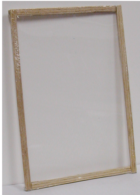
Figure 2.6: A photograph of a wooden frame 15.2 cm wide by 21.5 cm in length with a nitro cellulose membrane glued on the surface.
