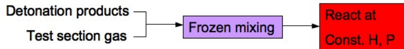
Figure 5.27: Homogeneous mixing ignition time model to characterize the time scale in which chemical reactions take place.
