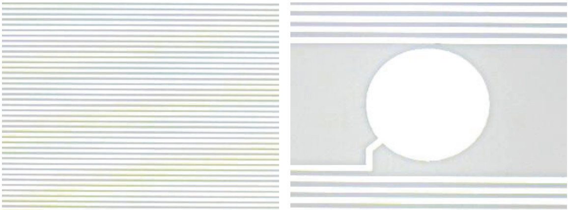
Figure 3-12. Results of titanium/platinum liftoff process. Liftoff of titanium and platinum from parylene is possible with at least 6 \mu\text{m} resolution.
