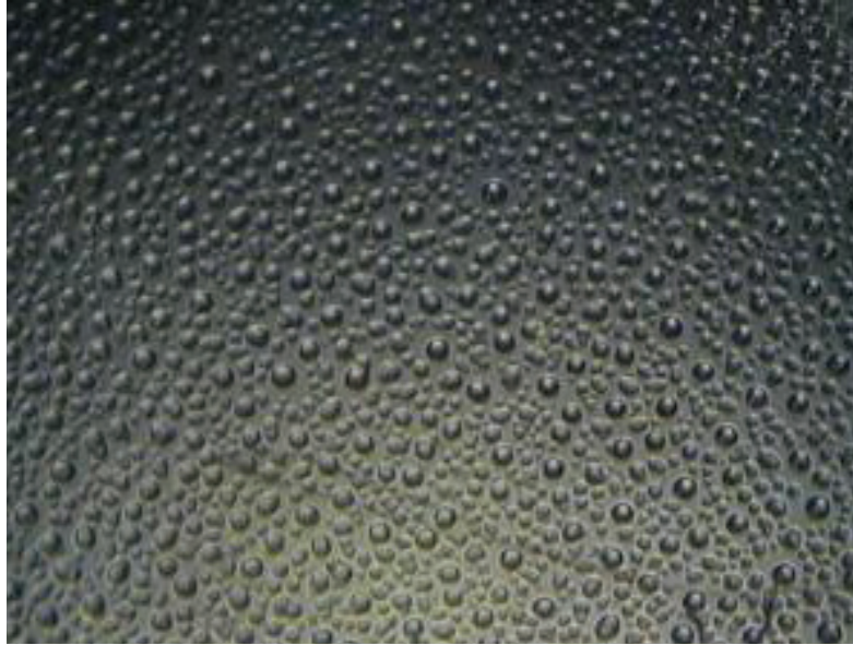
Figure 3-17. Unannealed parylene C sandwich structure after short accelerated-lifetime saline soak test. Interfacial delamination is clearly discernable.
