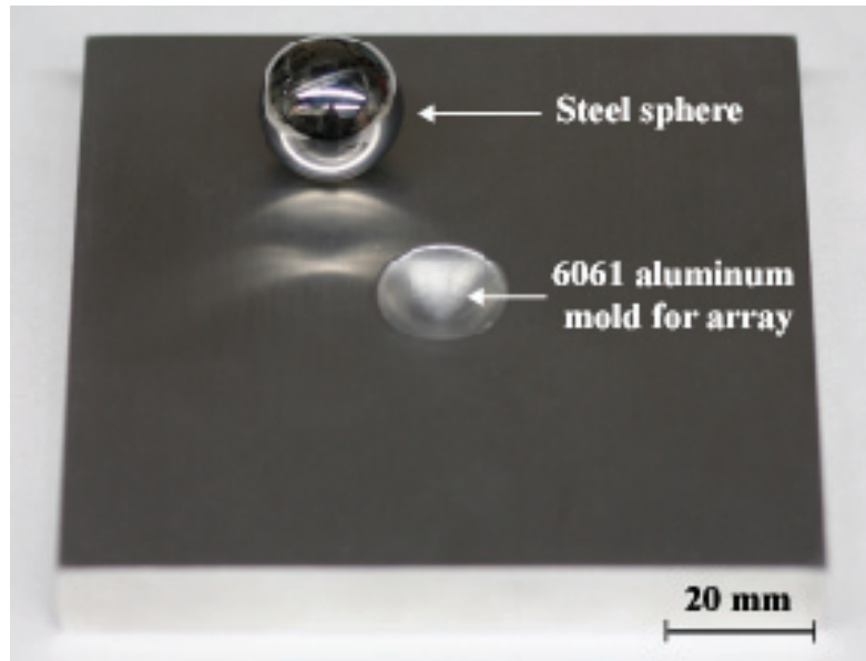
Figure 3-21. Custom heat-forming mold for chronic canine retinal implants.
