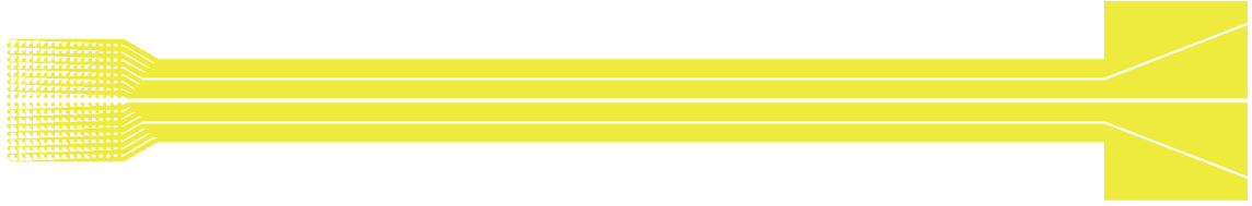
Figure 3-13. Approximately 50 mm long electrode array design.
