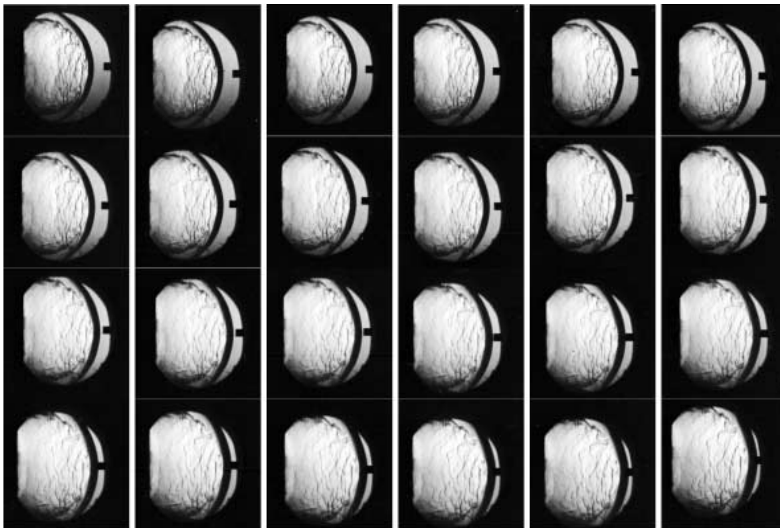
Stoichiometric hydrogen-oxygen mixtures with varying initial pressure, Shot 1195, P_I = 50 kPa
