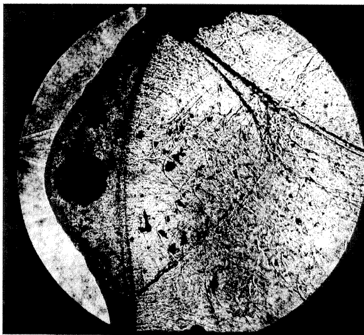
Figure B.37: Shot 1023 Shadowgraph: 2\text{H}_2 + \text{O}_2 + 3\text{N}_2 at 0.831 bar, 2330 m/s.
