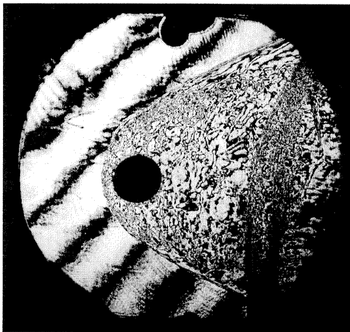
Figure B.15: Shot 1012 Interferogram: 2\text{H}_2 + \text{O}_2 + \text{N}_2 at 0.250 bar, 2500 m/s.
