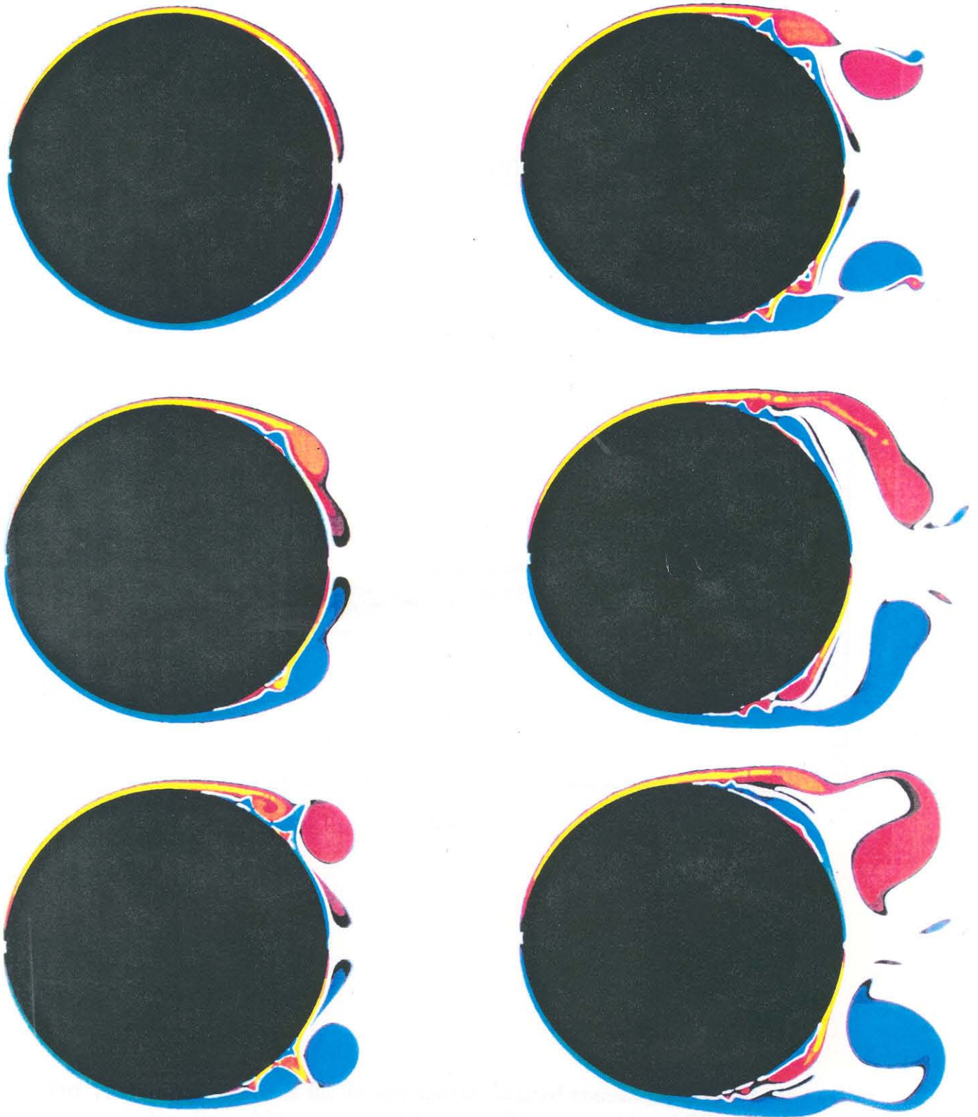
FIG. 7.30 Vorticity field of an impulsively started circular cylinder at Re = 9500 . ( T = 1.0, T = 2.0, T = 2.5, T = 3.0, T = 3.5, T = 4.0 : Frames are from top to bottom and left to right).
