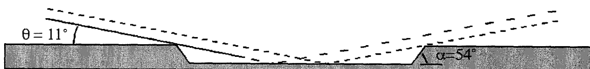
Figure N2-4: The focusing beam bouncing in and out of the cavity formed in the silicon wafer.
