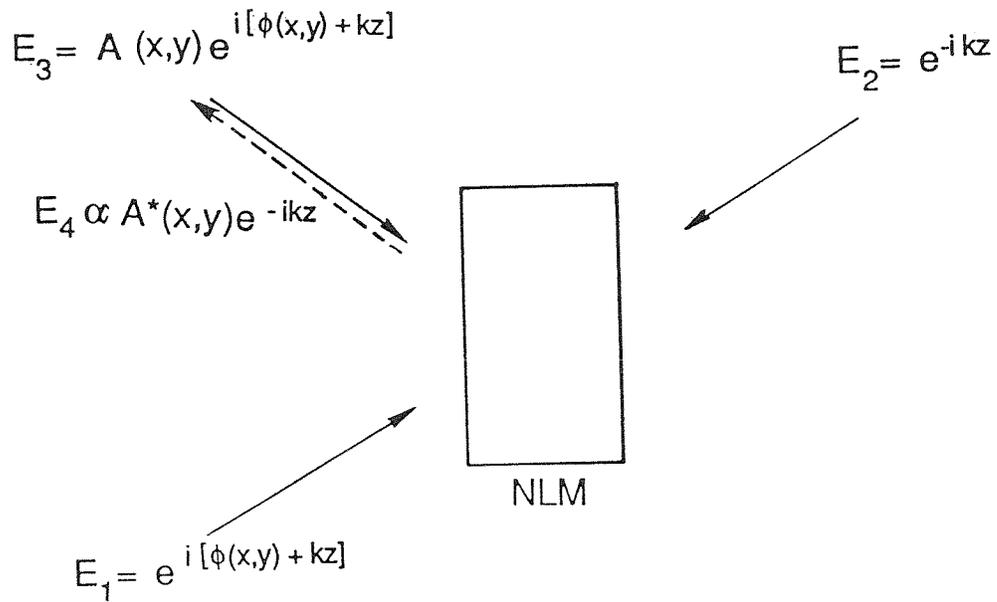
Fig. 1-5: Four-wave mixing configuration of phase conjugation, where waves 1 and 2 are the counterpropagating pump beams, 3 is the incident signal beam, and 4 is the phase conjugate.
