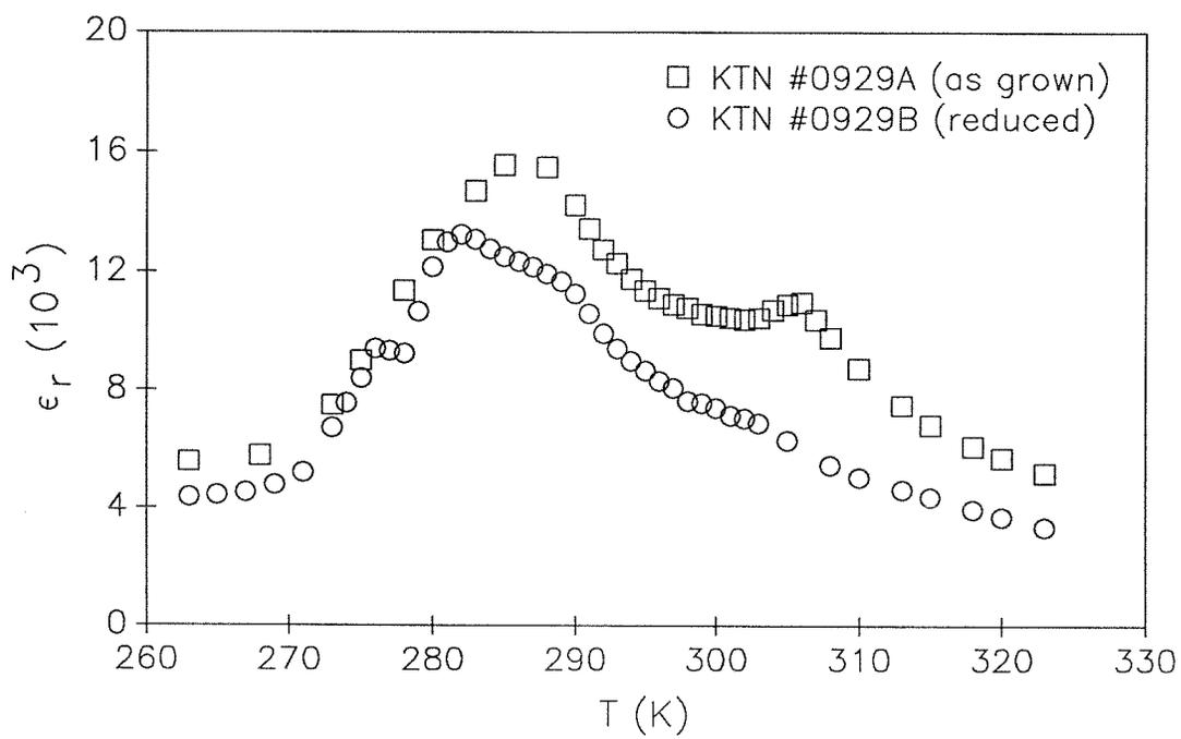
**Fig. 4-5:** Shift in the phase transition temperature of KTN:Cr,Fe (sample A, #929A) after reduction.
