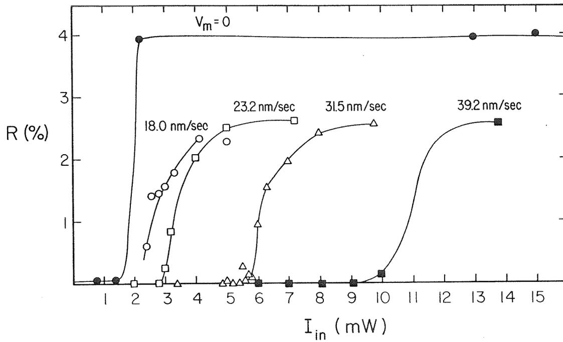
Fig. 7-7: Reflectivity as a function of beam intensity for the thresholding semilinear phase conjugate mirror.
