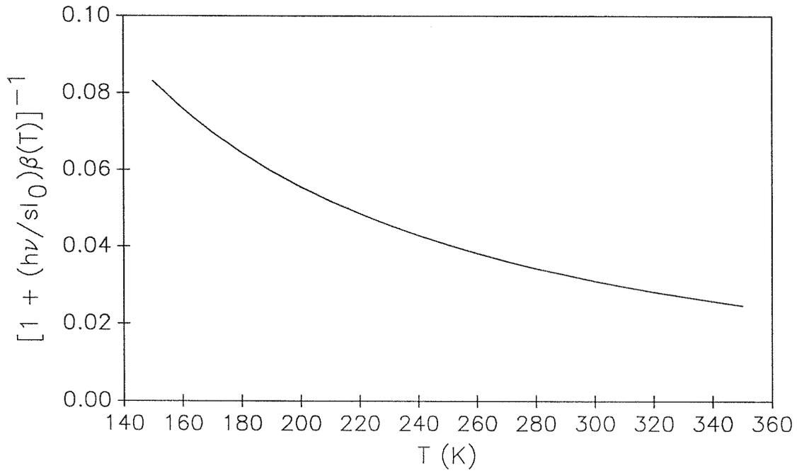
Fig. 5-11: Temperature dependence of the dark conductivity factor in the equations for gain and response time,  $[1 + (h\nu/sI_0)\beta(T)]^{-1}$ , from 150 to 350 K for  $E_t = 0.02$  meV and  $h\nu/sI_0 = 60$ .
