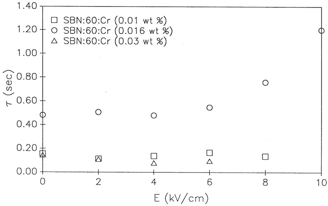
Fig. 6-11: Response time of the SBN:60:Cr crystals with an external DC field. The time constant remains within an order of magnitude of its value at  $E_0 = 0$ .
