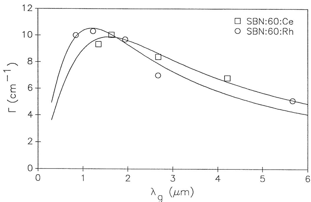
**Fig. 5-2:** Coupling constant as a function of grating wavelength for Rh-doped SBN:60 and Ce-doped SBN:60. The lines are the best fits of the expected gain coefficient as a function of grating period.
