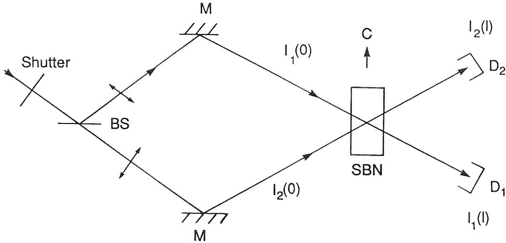
**Fig. 5-1:** Configuration for the two-beam coupling experiment used to characterize the SBN crystals. The beam polarization was in the same plane as the  $c$  axis.  $I_1(0) + I_2(0)$  was approximately  $0.25 \text{ W/cm}^2$ , with  $I_2(0) \ll I_1(0)$  to avoid pump depletion.
