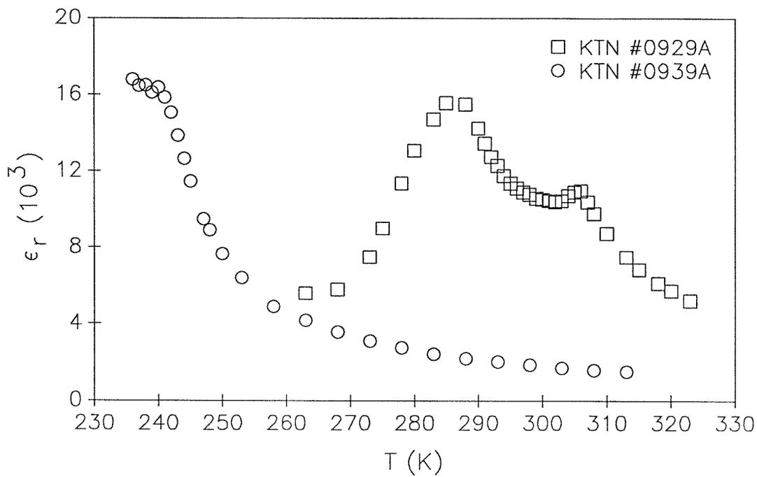
**Fig. 4-1:** Relative dielectric constant  $\epsilon_r$  of as-grown KTN:Cr,Fe near the phase transition temperature.
