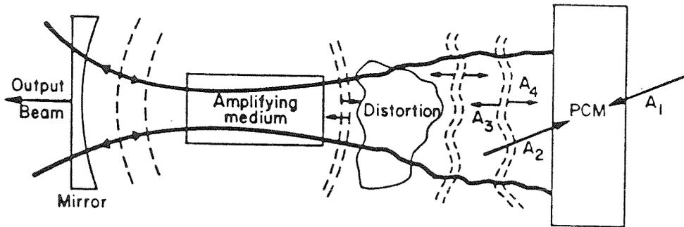
Fig. 1-4: Illustration of the distortion correction property of phase conjugate mirrors, where the phase conjugate reflection back through the distortion is the original undistorted beam.
