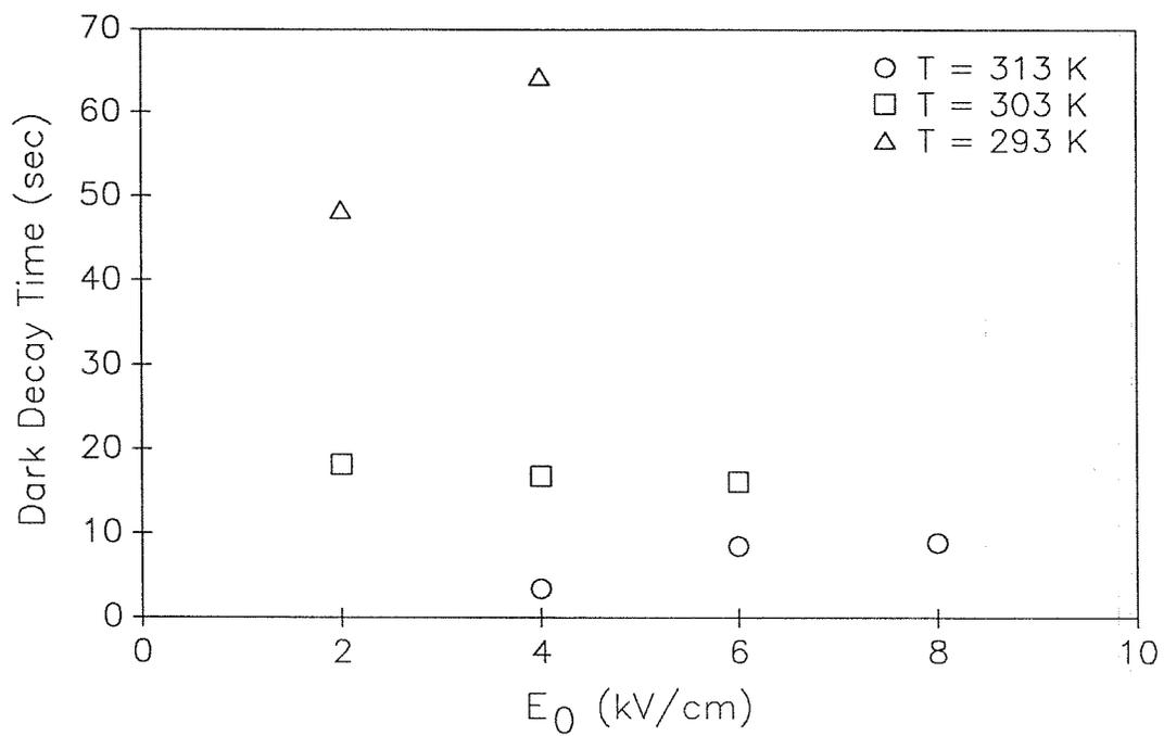
Fig. 4-7: Dark decay time of the reduced KTN:Cr,Fe crystal (sample A, #929A).
