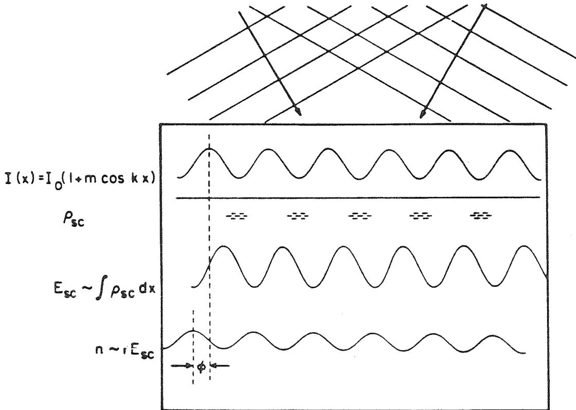
Fig. 1-1: Basic photorefractive mechanism, where the light interference pattern excites electrons from the donor sites to the conduction band where they drift and diffuse until retrapped in regions of low intensity. The electro-optic effect acts on the space charge field to produce the index modulation.
