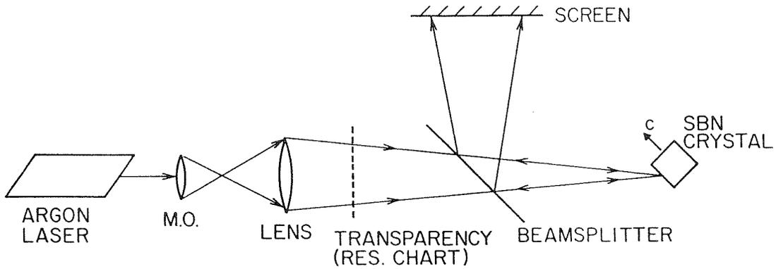
Fig. 7-1: Configuration of the self-pumped phase conjugate mirror using SBN used to study its reflectivity and distortion correcting properties.
