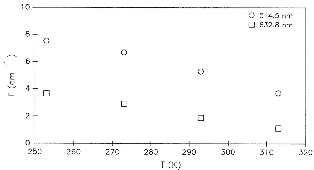
**Fig. 5-7:** Photorefractive two-beam coupling constant of Cr-doped SBN:60 at 514.5 and 632.8 nm incident wavelength with  $\lambda_g = 2.46 \mu\text{m}$ .
