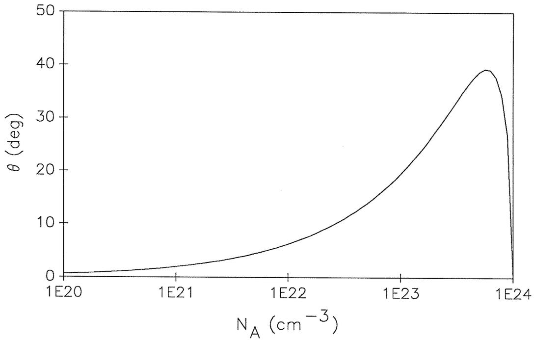
Fig. 6-5: Intersect angle required for the two incident beams in order to obtain the optimum grating period as trap density is varied from  $10^{20}$  to  $10^{24}$   $\text{m}^{-3}$ .
