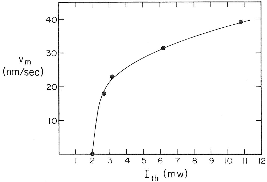
Fig. 7-8: Thresholding level as a function of grating velocity.
