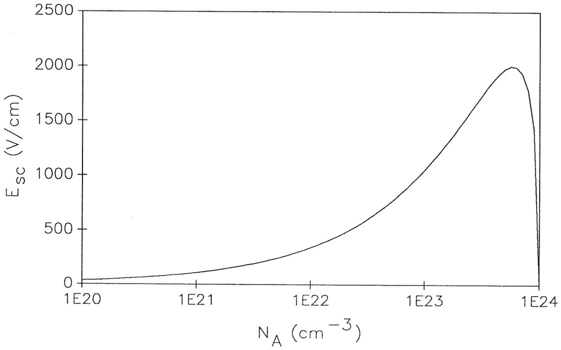
Fig. 6-4: Space charge field at the optimum grating period as a function of trap density, showing a  $\sqrt{N_A}$  dependence for  $N_A < N_0$ .
