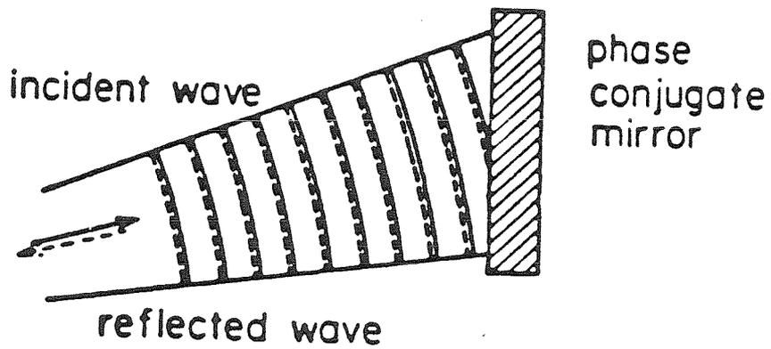
Fig. 1-3: The difference between reflections from a regular mirror (top), where the distorted wavefronts are merely reversed, and a phase conjugate mirror (bottom), where the incident wavefronts are retraced.
