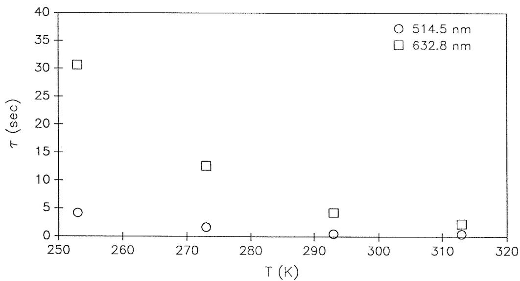
**Fig. 5-8:** Response time of the Cr-doped SBN:60 crystal at the two incident wavelengths.
