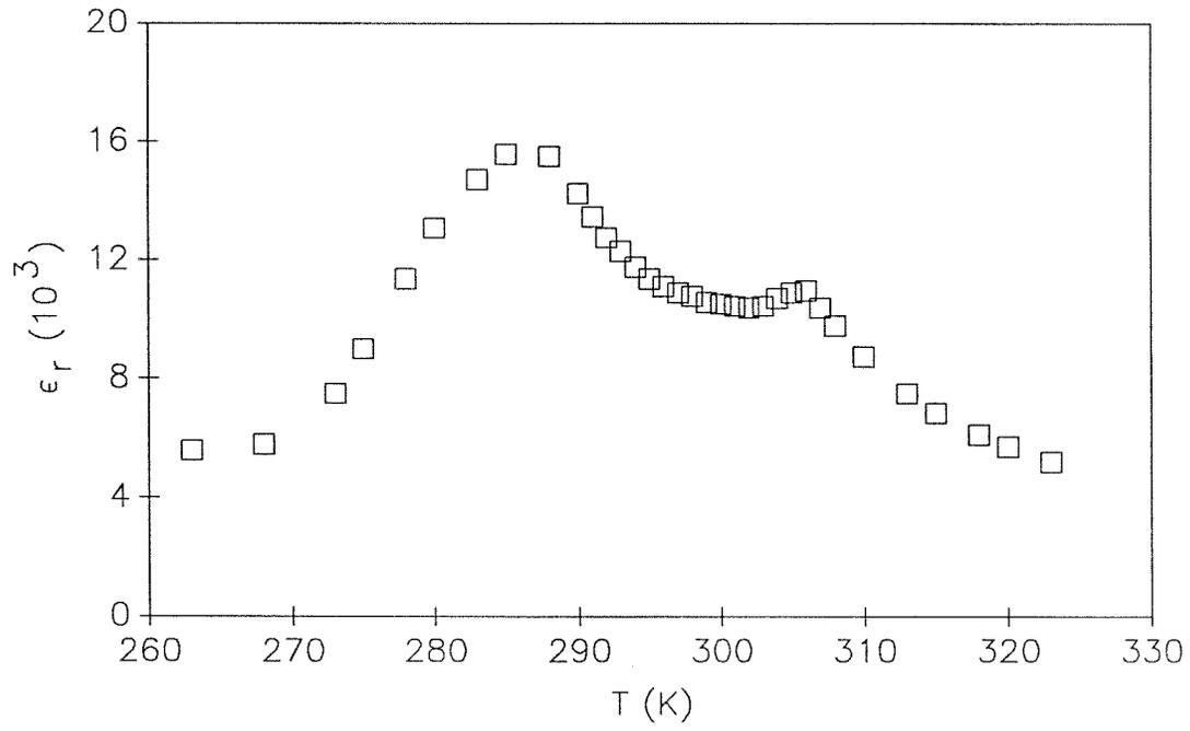
**Fig. 3-4:** Relative dielectric constant of KTN:Cr,Fe showing the sharp discontinuity in  $\epsilon$  at the ferroelectric to cubic phase transition temperature.
