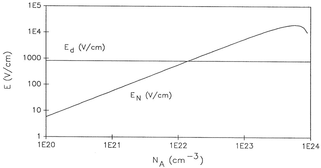
**Fig. 6-2:** Diffusion field  $E_d$  and maximum space charge field  $E_N$  as a function of trap density  $N_A$  for a fixed grating period  $\lambda_g = 2 \mu\text{m}$ .
