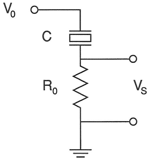
**Fig 3-3:** Method used to measure the low frequency capacitance and therefore determine the dielectric constant of the crystal. The conditions used were  $R_0 = 1$   $K\Omega$  and  $\nu = 10$  Hz.
