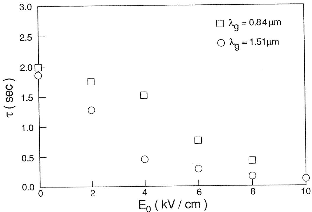
Fig. 6-13: Experimental response time of the SBN crystal for  $\lambda_g = 1.51$  and  $0.84 \mu\text{m}$ , which decreased from 2 sec at  $E_0 = 0$  to approximately 0.1 sec for  $E_0 = 10$  kV/cm.
