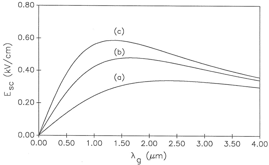
**Fig. 6-1:** Space-charge field as a function of grating period for (a)  $N_A = 10^{22} \text{ m}^{-3}$ , (b)  $N_A = 2 \times 10^{22} \text{ m}^{-3}$ , and (c)  $N_A = 3 \times 10^{22} \text{ m}^{-3}$ .
