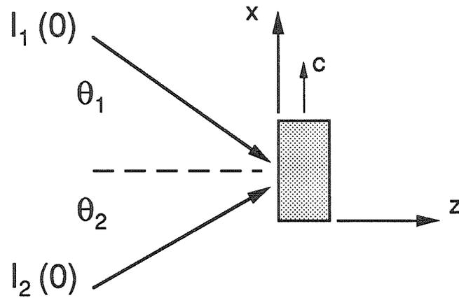
**Fig. 2-1:** Experimental geometry for wave mixing in photorefractive crystals, where waves 1 and 2 have incidence angles from the normal of  $\theta_1$  and  $\theta_2$ , respectively.
