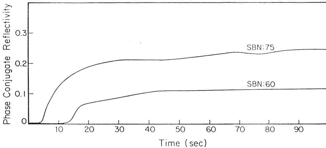
Fig. 7-2: Phase conjugate reflectivities as a function of time for the Ce-doped SBN:60 and SBN:75 phase conjugators. Pump beam power density was approximately  $1.5 \text{ W/cm}^2$ .
