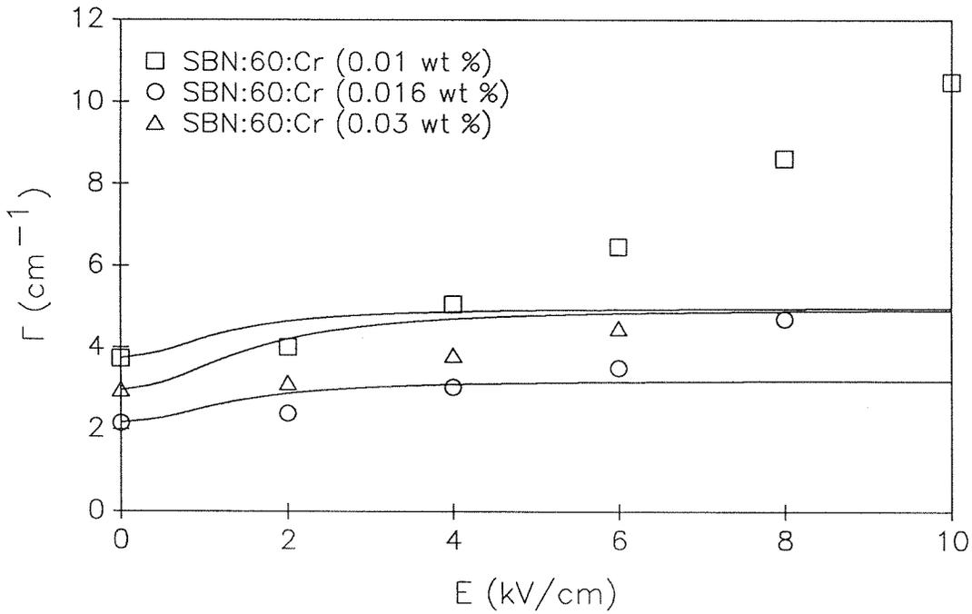
Fig. 6-10: Photorefractive two-beam coupling constant of the three Cr-doped SBN:60 samples as an external DC field from 0 to 10 kV/cm was applied. The increase in  $\Gamma$  beyond that predicted by theory may be the result of changes in some material parameters at high  $E_0$  or the effects of beam intensity depletion due to fanning. The  $E_0 = 0$  value of  $\Gamma$  was used as the initial operating point.
