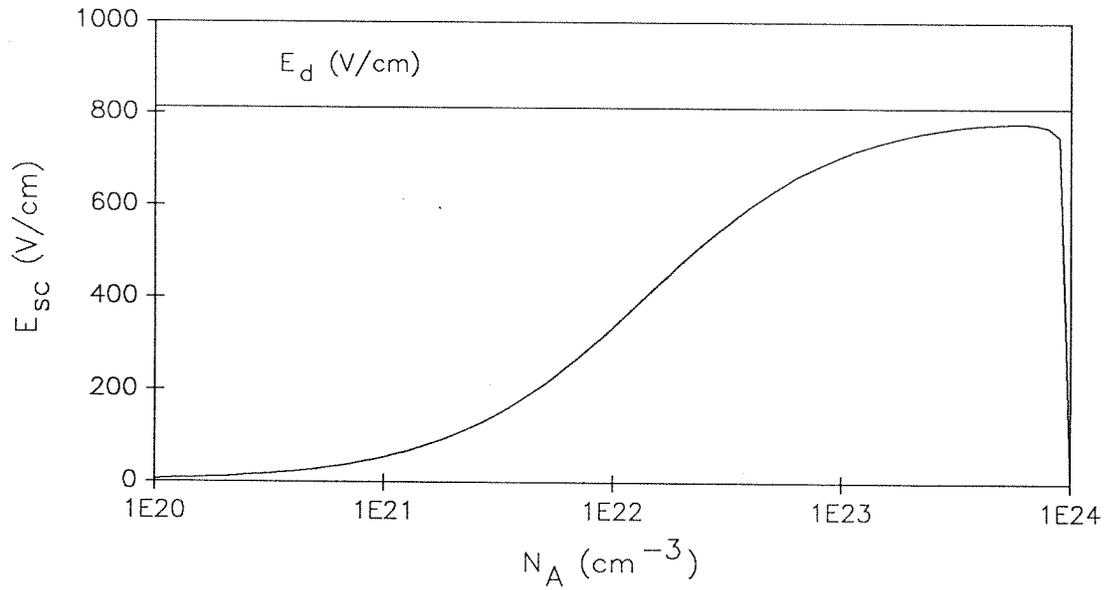
**Fig. 6-3:** Space charge field as a function of trap density for a fixed grating period.
