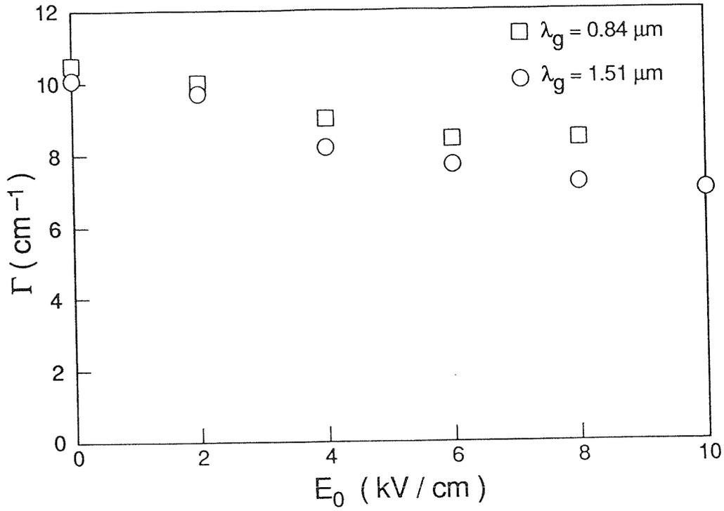
Fig. 6-12: Measured gain coefficient as a function of  $E_0$  for  $\lambda_g = 1.51$  and  $0.84 \mu\text{m}$ .
