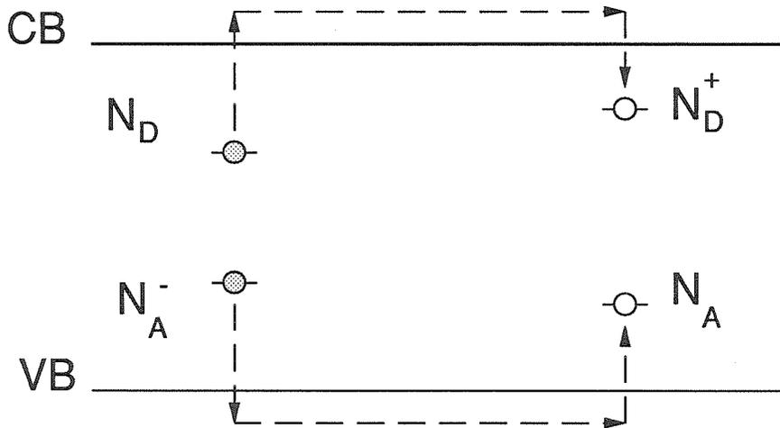
**Fig. 2-2:** Band transport process, where electrons are photoexcited from donor sites  $D$  into the conduction band, where they drift and diffuse until re-trapped in sites  $D^+$ . A similar process may be present for holes as well.
