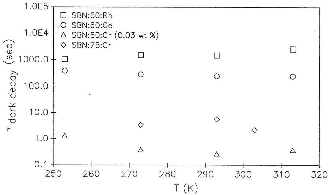
**Fig. 5-15:** Dark decay times for various SBN:60 and SBN:75 crystals, measured using a low intensity, vertically polarized He-Ne laser Bragg-matched to the photorefractive gratings, for  $I_0 = 0.5 \text{ W/cm}^2$  and  $m = 1$ .
