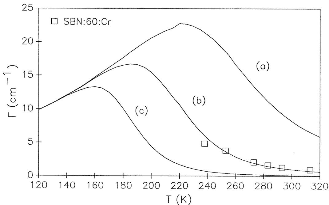
**Fig. 5-12:** Theoretical temperature dependence of the gain for different dark conductivities. The experimental points in the plot were obtained using the 0.01 wt. % Cr-doped SBN:60 crystal. The three cases illustrated are: (a) low dark conductivity,  $A = (h\nu/sI_0)\beta_0 = 6$ ; (b) best fit of the experimental points,  $A = 60$ ; and (c) high dark conductivity,  $A = 600$ .
