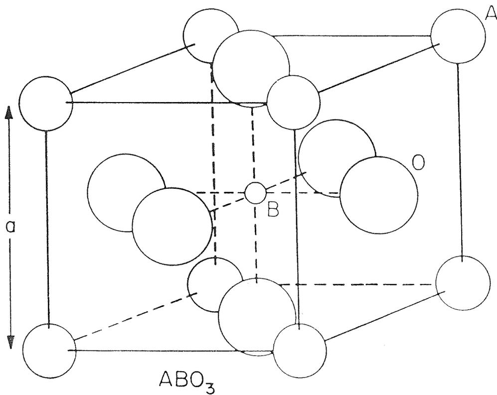
Fig. 3-1: Perovskite crystal structure with A at the corners, B at the body centers, and O at the face centers.
