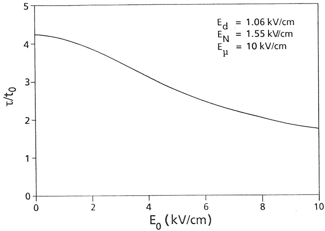
Fig. 6-9: Expected response time as a function of applied field for  $E_d = 1.06$  kV/cm,  $E_N = 1.55$  kV/cm, and  $E_\mu = 10$  kV/cm, showing  $\tau/t_0$  approaching unity for large applied field  $E_0$ .
