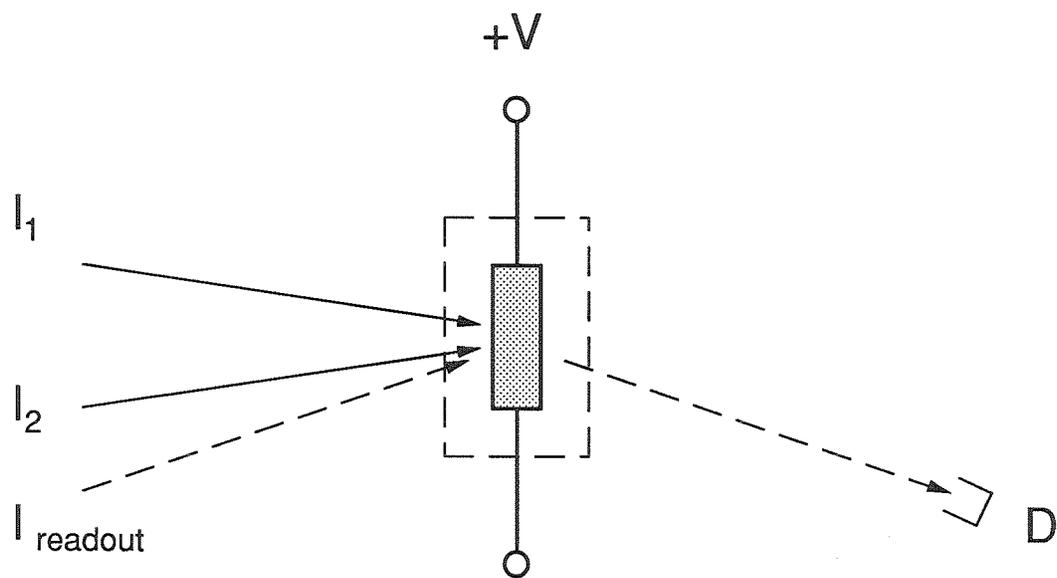
**Fig. 3-6:** Configuration used to measure the diffraction efficiency of KTN.
