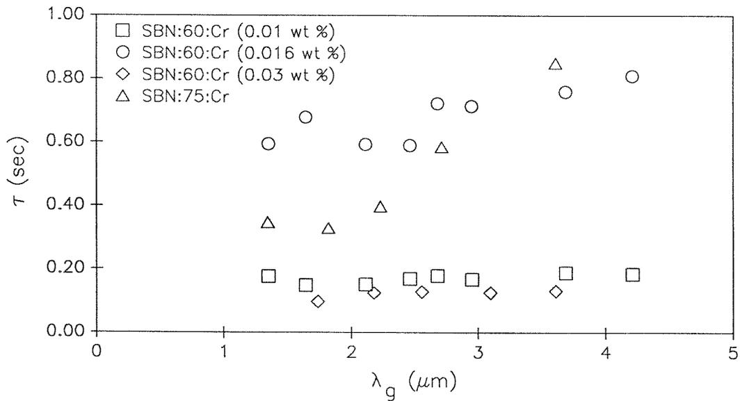
Fig. 5-5: Response time of the three Cr-doped SBN:60 and Cr-doped SBN:75, showing the almost order of magnitude increase in the speed of response over Ce or Rh doping.
