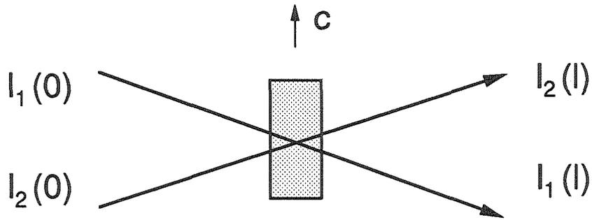
Fig. 1-2: Photorefractive two-beam coupling resulting in beam amplification of  $I_2$  and depletion of energy from  $I_1$ .
