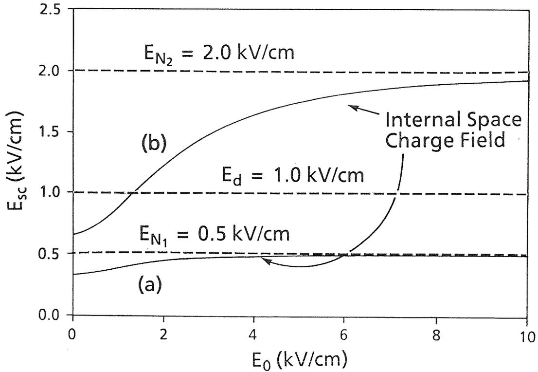
Fig. 6-8: Expected space-charge field as a function of the applied DC field for (a)  $E_N < E_d$ , with  $E_N = 0.5$  kV/cm and  $E_d = 1.0$  kV/cm, and (b)  $E_N > E_d$ , with  $E_N = 2.0$  kV/cm and  $E_d = 1.0$  kV/cm. Note that the space-charge field approaches  $E_N$  for large  $E_0$ .
