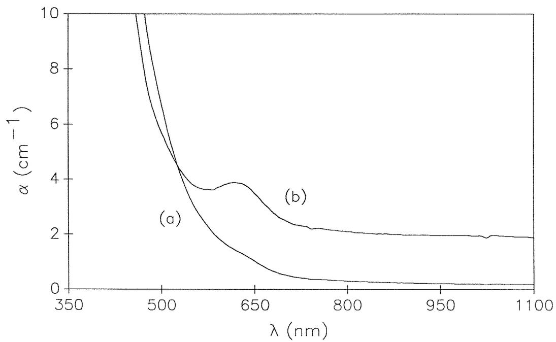
**Fig. 3-2:** Absorption spectrum of (a) as-grown KTN:Cr,Fe and (b) same KTN:Cr,Fe after reduction of  $\text{Cr}^{6+}$  by heating in Ar.
