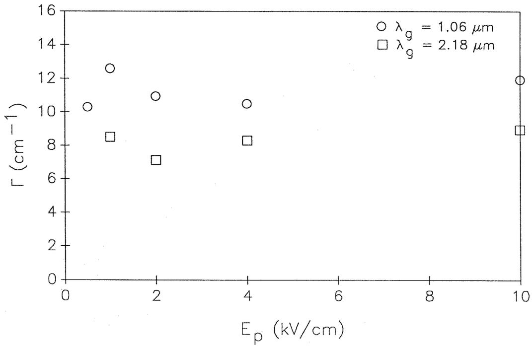
**Fig. 5-6:** Two-beam coupling constant of Rh-doped SBN:60 as a function of poling voltage from 0.5 to 10 kV/cm.
