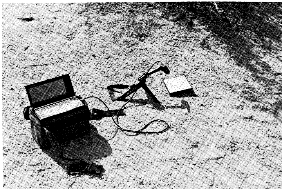
Figure 60: Photograph of Analytic Spectral Devices Personal Spectrometer 2 in operation in the Manix Basin.
