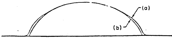
FIG. 2. Comparison of Pierrehumbert's' solution (a) and present solution (b) for vortices of the same width.
