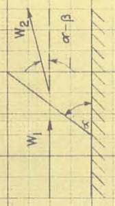
CHANGE IN DIRECTION OF FLOW THROUGH OBLIQUE CONDENSATION SHOCK.
