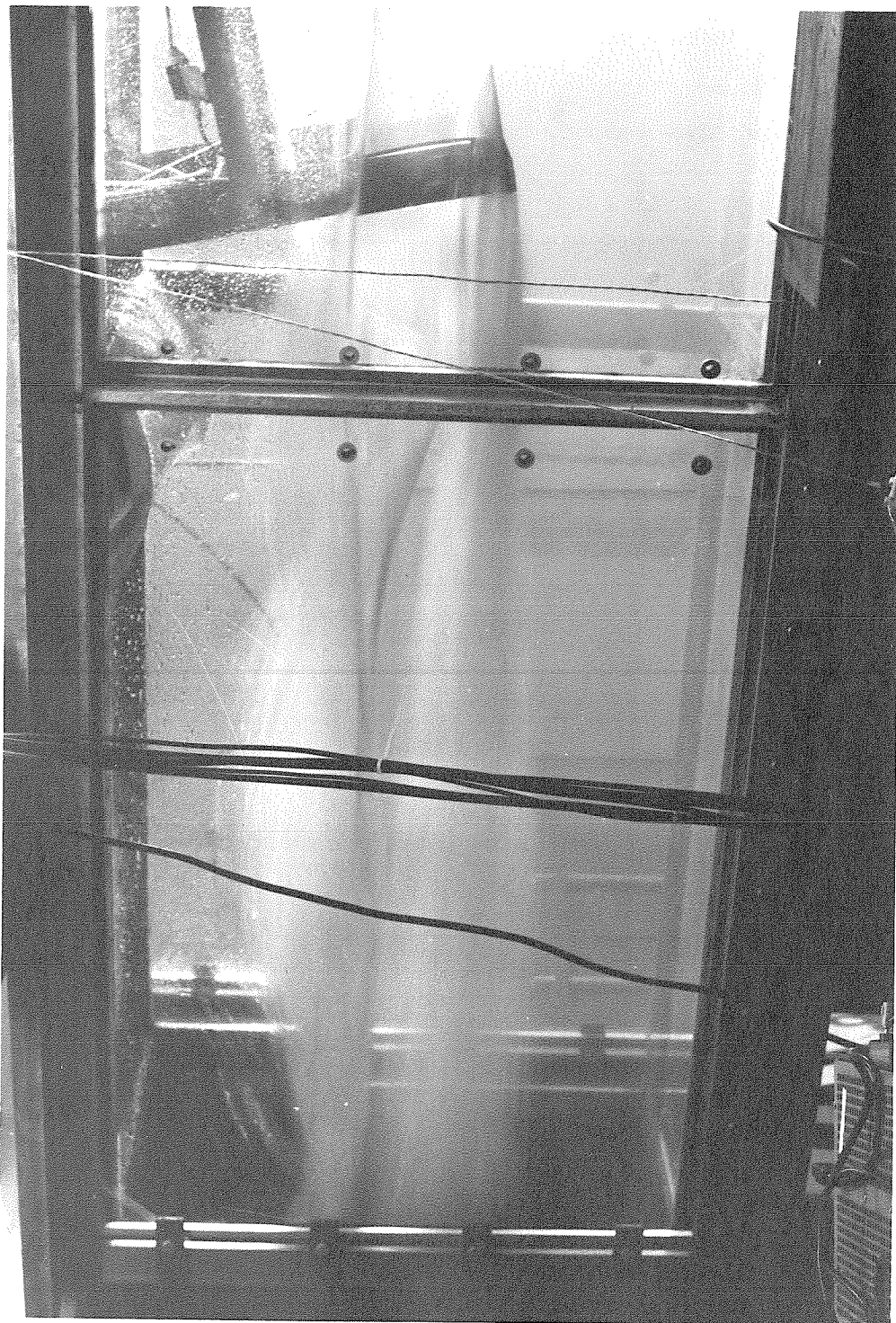
FIG. 15 VENTILATED CAVITY IN THE F.S.W.T.
