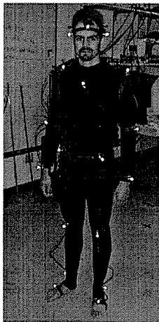
Figure 6.1: Mocap suit: In order to capture the movement of the human body in 3-D, 18 light-bulb markers are placed on the major joints of the body.
