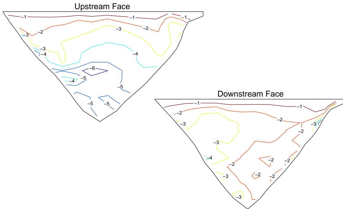
Figure C.24: Maximum compressive cantilever stresses (MPa) computed during a nonlinear analysis with the Northridge earthquake input (method 2)
