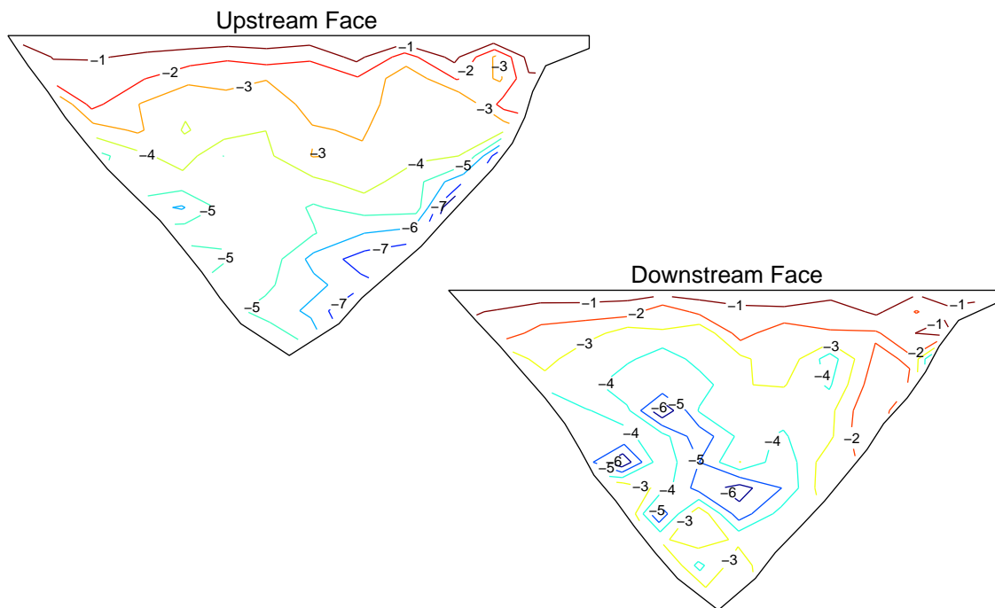
Figure C.28: Maximum compressive cantilever stresses (MPa) computed during a nonlinear analysis with the Northridge earthquake input (method 4)
