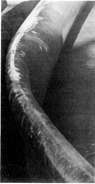
(a) Propagating buckle on a 12 in. pipe.
