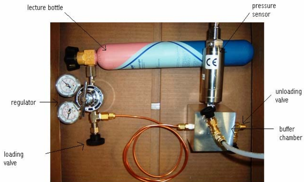
Figure 3.1. Pressure-handling module (without the meter).
