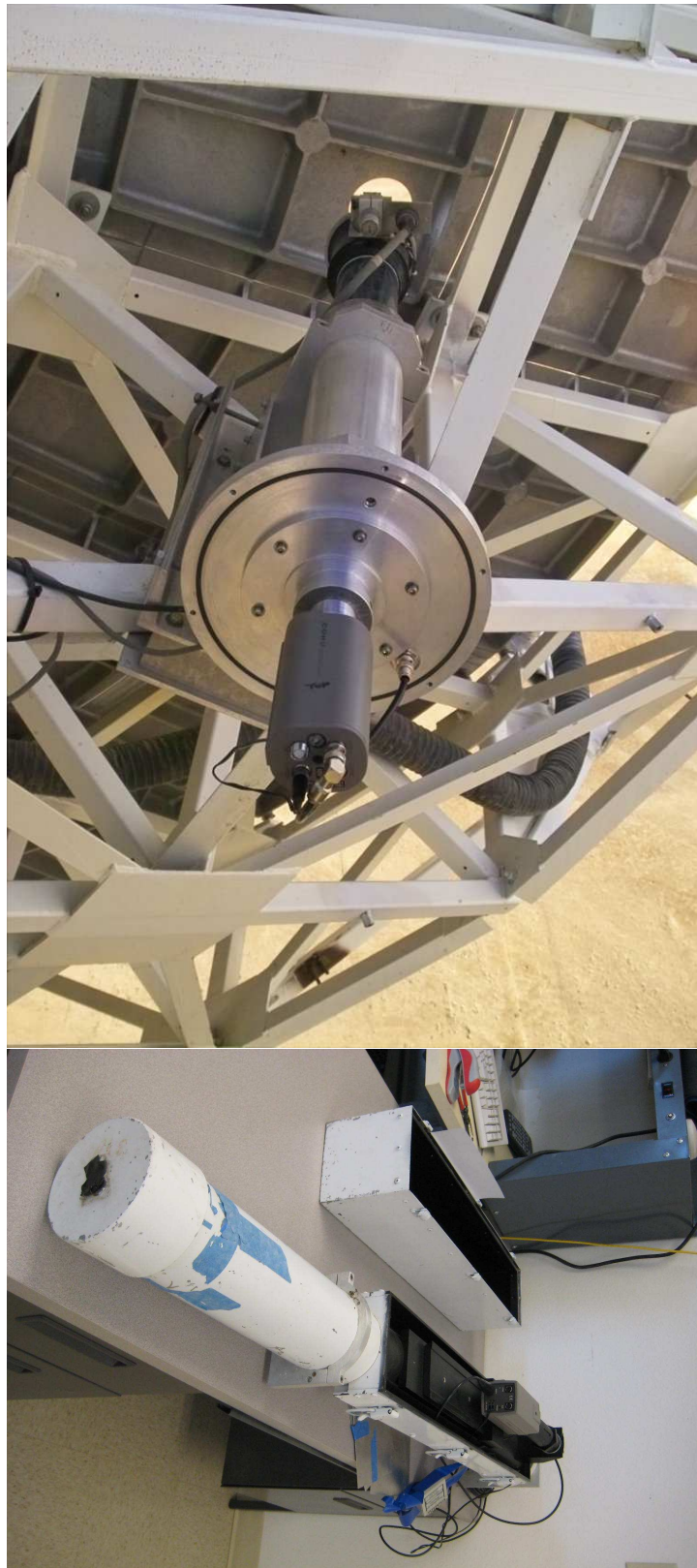
Figure B.1 The top panel shows the optical telescope used on the 6-m antennas. In the bottom panel, the 6-m antenna optical telescope is shown. The 10-m antenna telescope aperture is located behind the white cap on the left side of the image. The 6-m optical telescope is shown mounted to the antenna.
