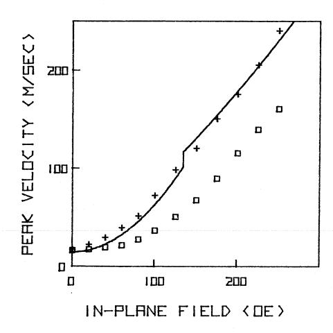
Fig. (4.5). Peak velocity as a function of in-plane field magnitude with an in-plane field direction ( $\square$ ) along or (+) opposed to the direction of the stray field at the implanted surface.
