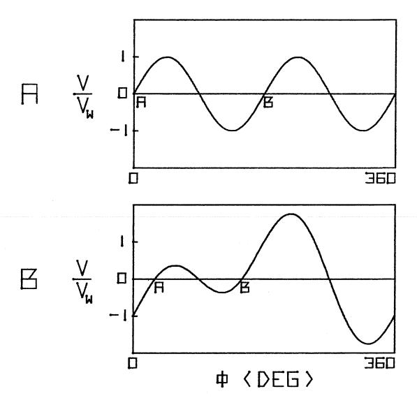
Fig. (2.8). The velocity vs.  $\phi$  characteristic for (a) H $_y$  = 0 and (b) H $_y$  = 4M. The velocity is normalized to the Walker peak velocity.
