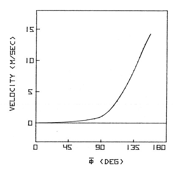
Fig. (E.4). Steady-state wall velocity as a function of average azimuthal angle.
