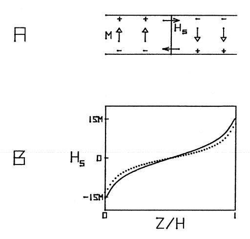
Fig. (2.4). (a) The orientation of the stray field  $H_S$  at a domain wall. (b) The magnitude of the stray field at the wall, as a function of position. The solid line is for an isolated wall while the dotted line is for a 5  $\mu$ m diameter bubble in a 4  $\mu$ m thick film.
