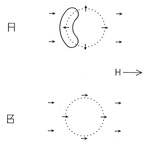
Fig. (3.3). Spin configuration in the implanted layer for an external in-plane field H much less than (a) and much greater than (b) the peak bubble stray field.
