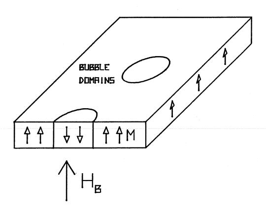
Fig. (1.1). Bubble domains in a thin ferromagnetic film, showing the direction of the magnetization  $\overline{M}$  and the applied bias field  $\overline{H}_{\underline{b}}$ .
