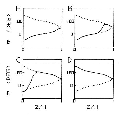
Fig. (2.10). The time evolution of the spin configuration during a pulse, showing qualitatively the nucleation, propagation and punch-through of a horizontal Bloch line.
