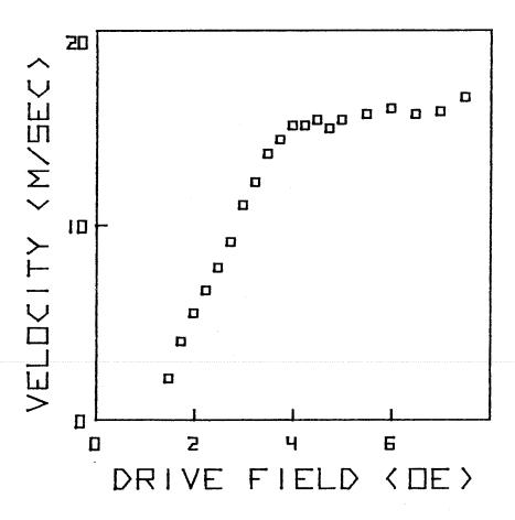
Fig. (4.2). Steady-state wall velcoity as a function of drive field.
