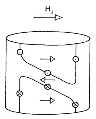
Fig. (E.2b). The location of the wall twist in a unichiral bubble for a 20 Oe in-plane field. The arrows show the direction of  $\overline{M}$ .
