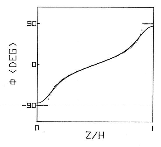
Fig. (2.5). The azimuthal angle of the spin orientation is plotted as a function of distance through the film thickness. The dotted line shows the magnetostatic minimum.
