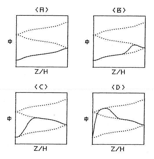
Fig. (4.9). The time evolution of the spin configuration of a  $\chi^-$  state when an expanding bias pulse is applied. The bottom film surface is implanted.
