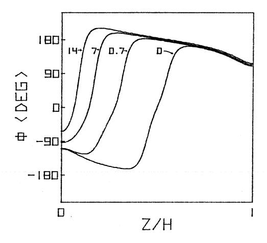
Fig. (E.3). Wall structure with steady-state velocity (m/sec) as a parameter. A 20 Oe in-plane field is applied opposite to the center spin.
