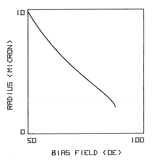
Fig. (A.1). Radius versus bias field for a bubble domain.
