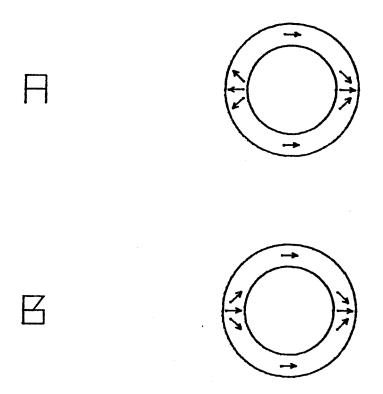
Fig. (3.5). The internal wall structure of (a) an S=1 bubble and (b) an S=0 bubble.
