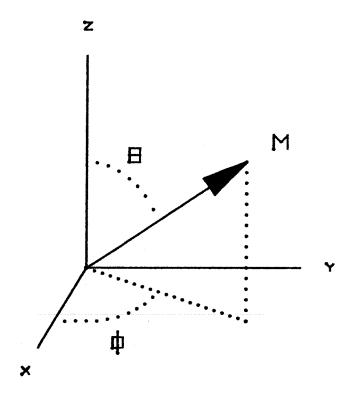
Fig. (2.1). The spherical polar coordinate system. The angles  $\theta$  and  $\phi$  specify the orientation of  $\overline{M}$  while (x,y,z) specifies the location in the material.
