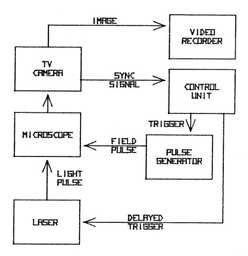
Fig. (C.1). Block diagram of the optical sampling microscope.
