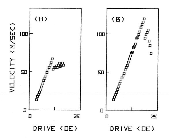
Fig. (4.4). Velocity as a function of drive field for a 150 Oe in-plane field applied (a) along or (b) opposed to the direction of the stray field at the implanted surface.
