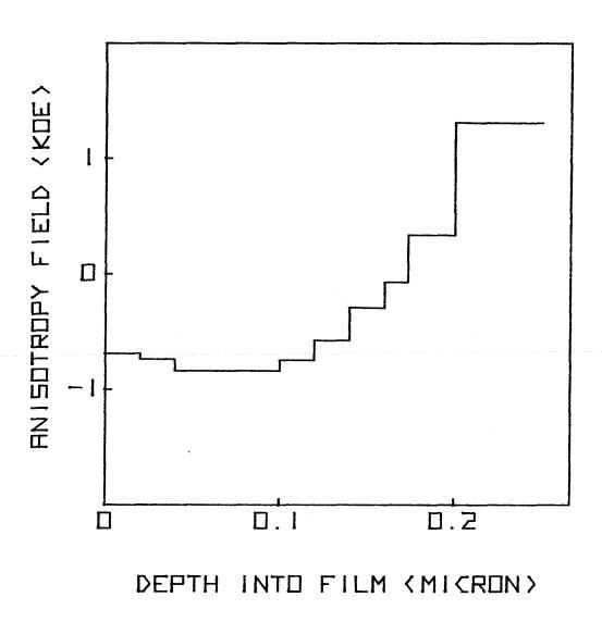
Fig. (3.1). The anisotropy field as a function of depth into the film.
