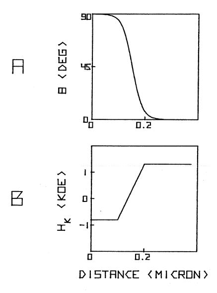
Fig. (3.2). (a) The polar angle of the magnetization is plotted as a function of distance into the film. The  ${\rm H}_{\rm k}$  distribution is shown in (b).
