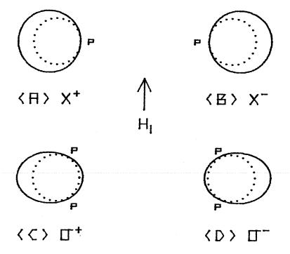
Fig. (4.7). The transient shape (solid line) of the four elementary bubble states during a test pulse with  $H_1$  = 10 Oe. The dotted line shows the equilibrium bubble position.
