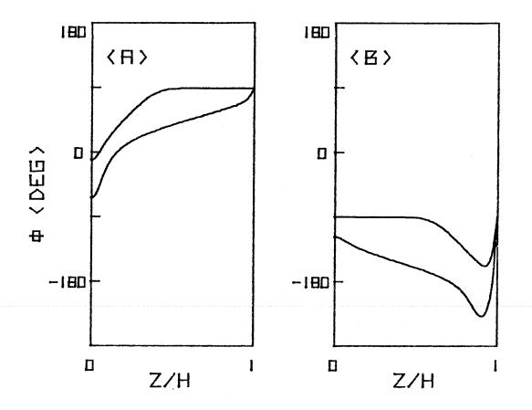
Fig. (4.6). The static (v=0) and dynamic ( $v=v_p$ ) spin cinfiguration in the wall for a 150 Oe in-plane field applied along (a) and opposite (b) to the direction of the stray field at the implanted surface.
