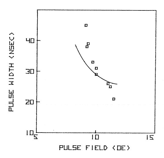
Fig. (E.6). The pulse width required to produce a  $\chi$ -to- $\sigma$  state switch as a function of pulse amplitude, for a 20 Oe in-plane field.
