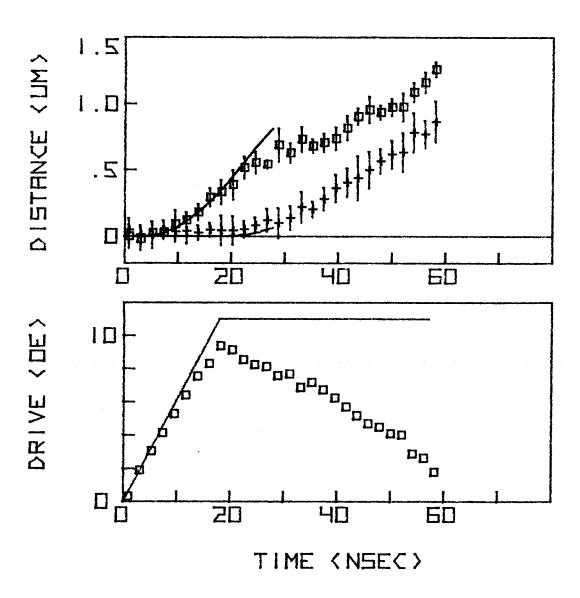
Fig. (E.5b). Displacement of the wall as a function of time after the start of an 11 Oe bias pulse. Also plotted is the instantaneous drive.
