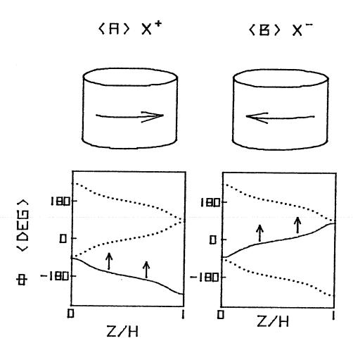
Fig. (4.8). The direction of spin precession in (a) a  $\chi^+$  and (b) a  $\chi^-$  bubble state. The HBL nucleates at opposite film surfaces for the two cases.
