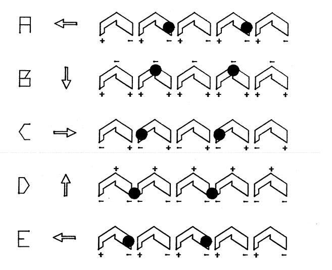
Fig. (1.3). Movement of the bubbles through a shift register. The arrows indicate the direction of the rotating field.
