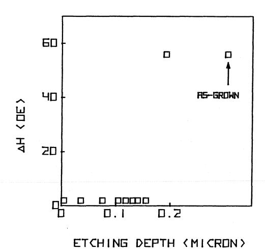
Fig. (3.6). The spread in collapse fields for bubbles in a series of etched films is plotted as a function of etching depth.
