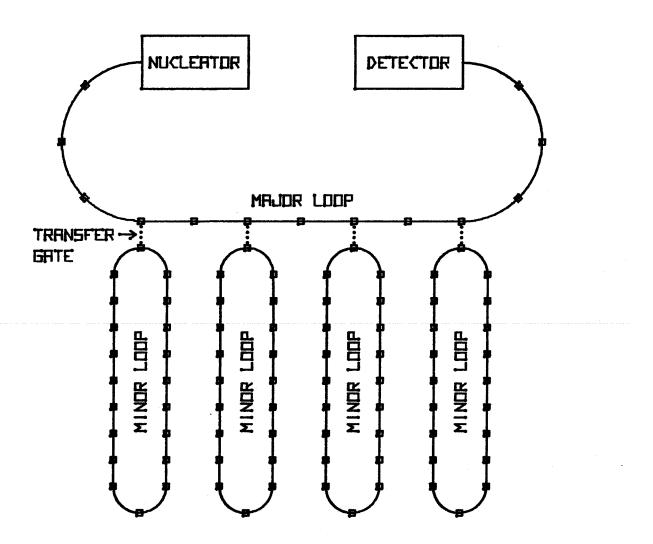
Fig. (1.2). Organization of a bubble device chip.
