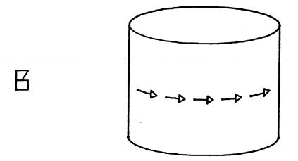
Fig. (1.4). (a) The orientation of spins through a Bloch wall.
