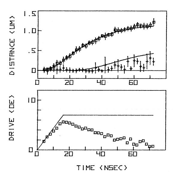
Fig. (E.5a). Displacement of the wall as a function of time after the start of a 7 Oe bias pulse. Also plotted is the instantaneous drive.
