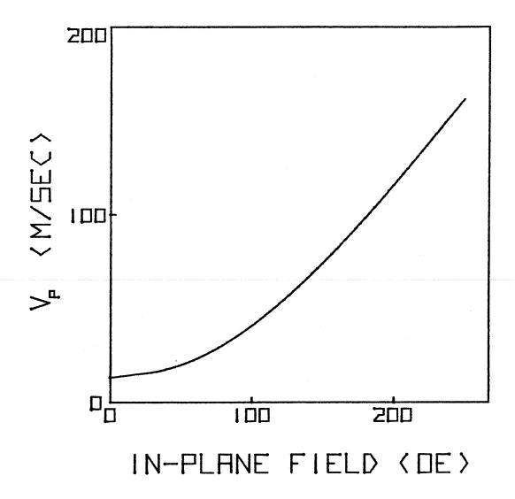
Fig. (2.9). Peak velocity as a function of in-plane field magnitude. The field is applied perpendicular to the wall.
