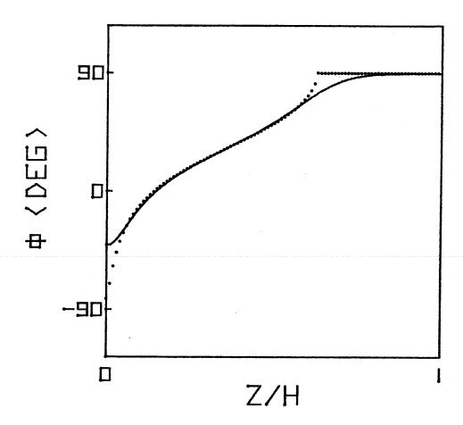
Fig. (2.6). The azimuthal angle of the spin orientation plotted as a function of position through the film thickness for  $H_y$  =  $2\pi M$  = 90 Oe. The dotted line shows the magnetostatic minimum.
