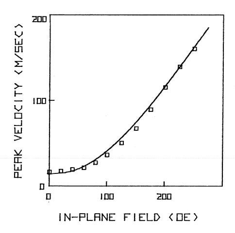
Fig. (4.3). Peak steady-state wall velocity as a function of in-plane field applied perpendicular to the wall.
