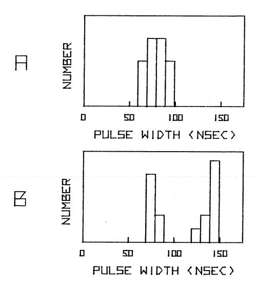
Fig. (4.12). The pulse width required to reconvert k-states back to the original unichiral states. The pulse was 5 Oe. In (a), the states were k=2 states. In (b), the states were a mixture of k=2 and k=4 states.
