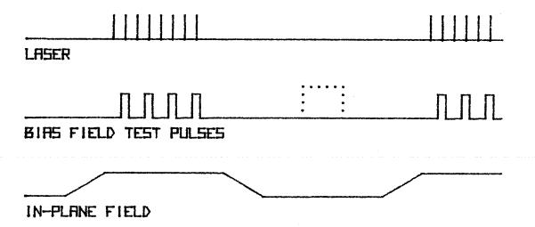
Fig. (D.1). Pulse sequence for the state identification experiment.
