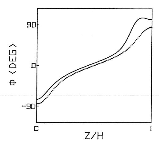
Fig. (2.7). The dynamic spin configuration at the peak steady-state wall velocity for zero in-plane field. The dotted line shows the static wall structure.
