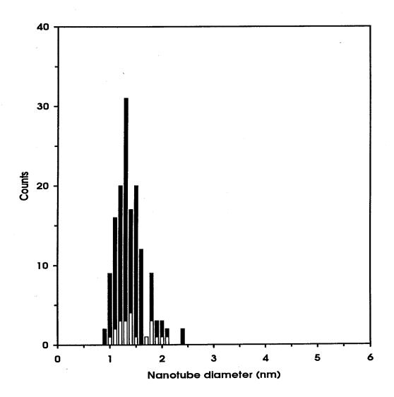
Figure 5.7: Single-layer carbon nanotube diameter distributions for samples made using 4 % Co from Co metal (black bars) and 2 % Co from Co oxide (white bars). All atomic percentages are with respect to the total carbon content of rod. The diameters of the tubes were obtained by measuring the distance between the most intense portions of the TEM image of the tube wall.
