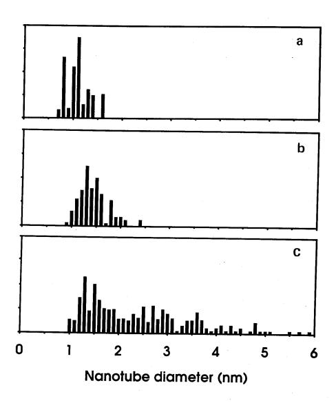
Figure 7.2: Diameter distribution of nanotubes produced via different methods: (a) Fe catalyst in an Ar/CH<sub>4</sub> atmosphere, adapted from Ref. [14]; (b) Co catalyst in He atmosphere, adapted from Ref. [4]; (c) Co catalyst with sulfur, about 4% each, adapted from Ref. [4].
