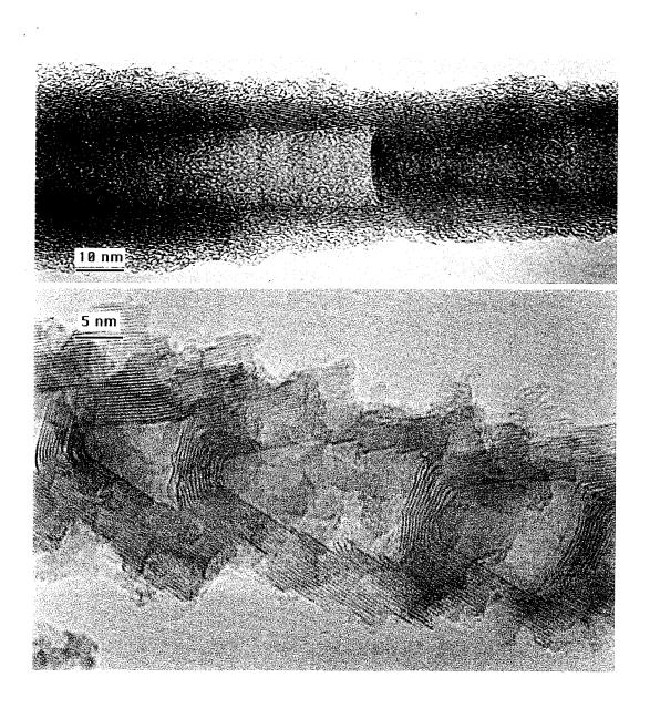
Figure 6.20: String of pyramidal shaped carbon beads, found in the rubbery soot.
