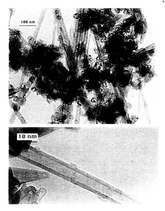
Figure 6.15: A typical composition of the central part of cathode deposit formed without catalyst.
