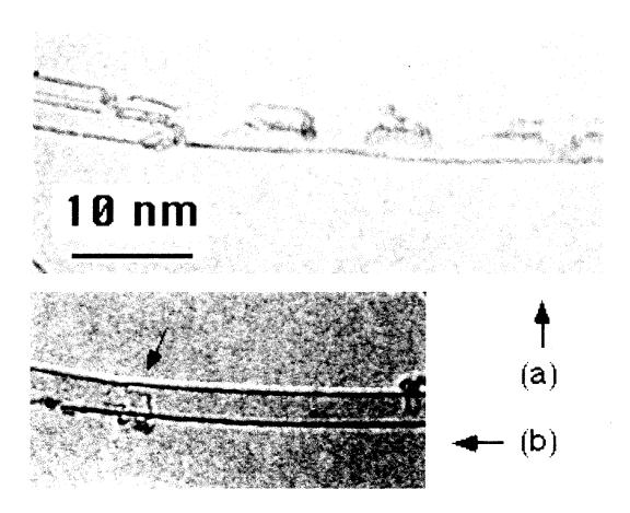
Figure 6.9: Breaking and forming carbon bonds of single-layer nanotube under electron beam heating. In (a) the tube was broken into sections, and in (b) the originally defective section was gradually healed.
