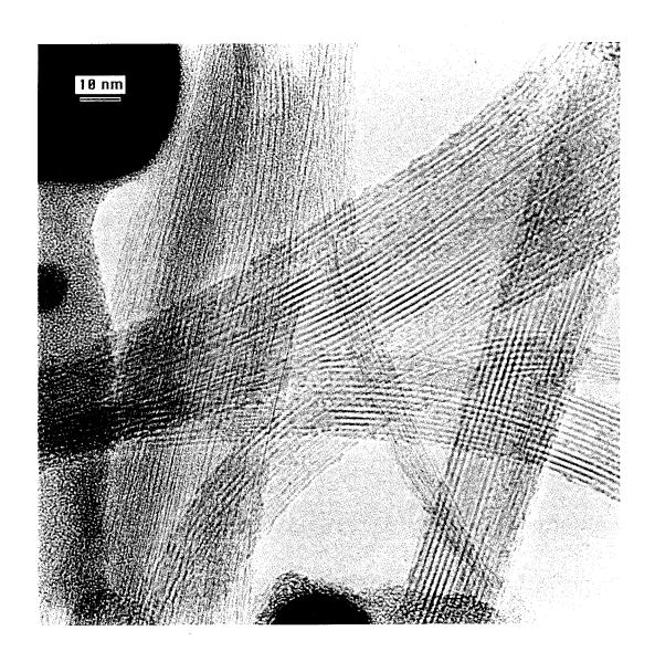
Figure 5.11: TEM of soot produced by vaporizing Co, Bi, and C in an arc. The large dark objects shown in the figure are pure Bi particles. The smaller spots are fcc Co crystals, as shown by EDS and high resolution TEM images.
