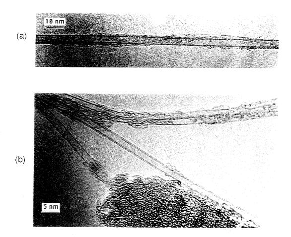
Figure 5.9: (a) High resolution image of a 3.6 nm diameter nanotube with a 1.3 nm tube spiraling around it. (b) Double-layer nanotube among single-layer nanotubes.
