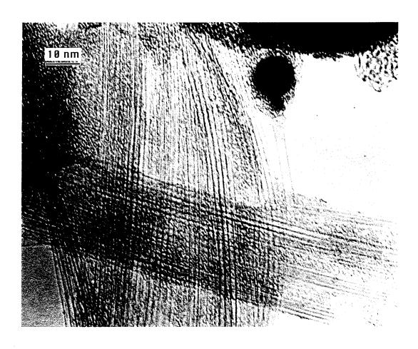
Figure 5.12: Bundles of single-layer carbon nanotubes produced with Co, Bi, and C. The 3 nm diameter tube is larger than any single-layer carbon nanotubes produced to date with Co alone.
