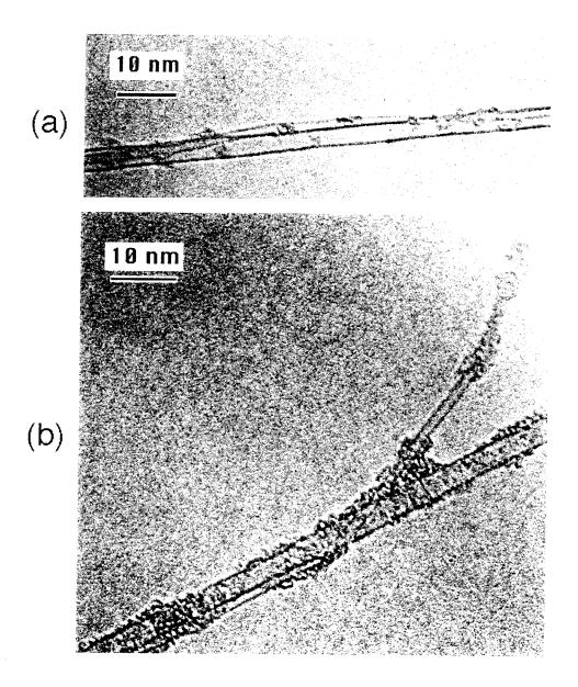
Figure 6.12: Two nanotubes coupled together. In (b) the tubes split at one end.
