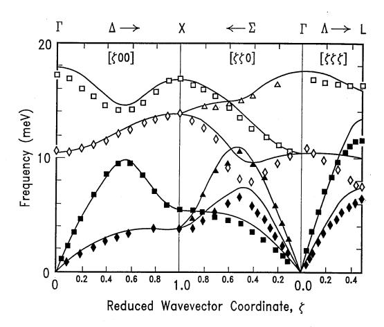
Figure 2.2: The phonon dispersion curves along  $[\zeta,0,0]$ ,  $[\zeta,\zeta,0]$ , and  $[\zeta,\zeta,\zeta]$  directions in AgBr at 4.4K (Ref. [19]). Solid curves are from Model II and the symbols are experimental values.
