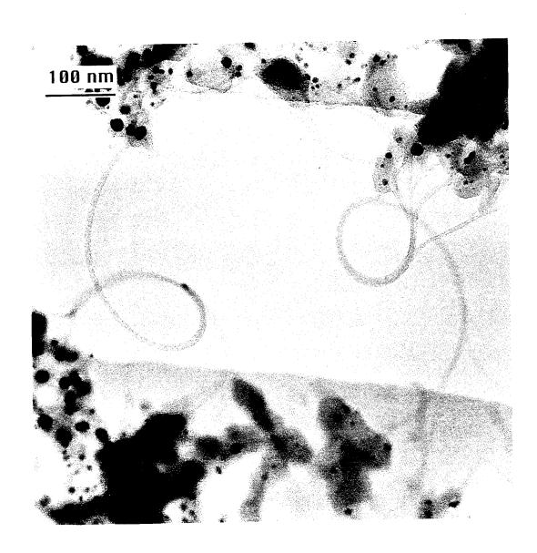
Figure 1.2: Transmission electron micrograph of single-layer carbon nanotubes produced by cobalt catalyst.
