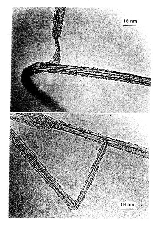
Figure 6.3: TEM of nanotubes showing (a) twisting and (b) bending.
