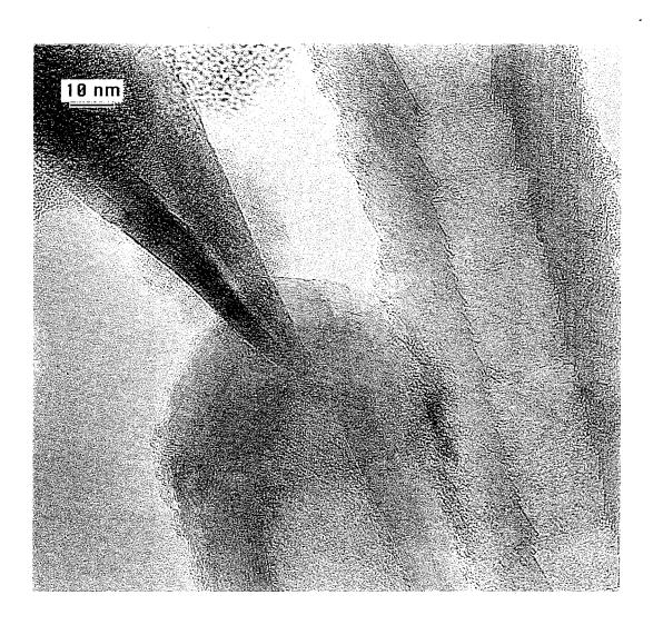
Figure 6.18: Carbon cone found in the rubbery soot, made with Co and S.
