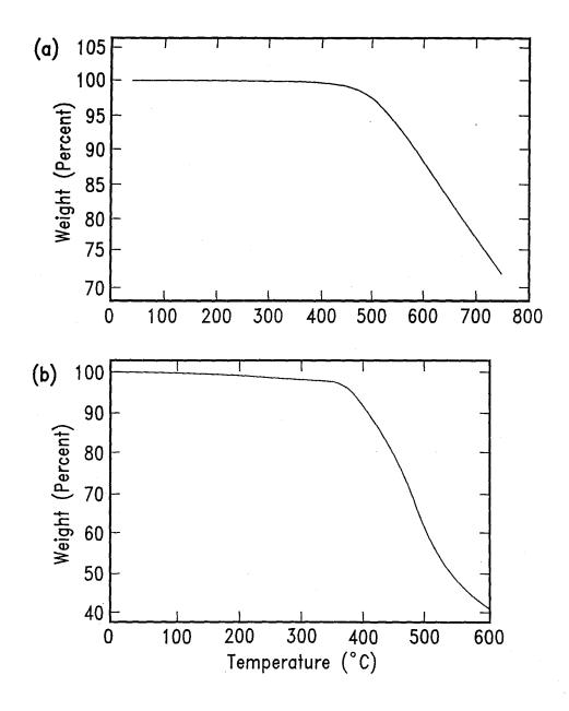
Figure 6.7: Thermogravimetric analysis of soot containing single-layer nanotubes made with (a) Co and, (b) Co and S. Samples were heated in  $N_2$  at the heating rate of 10  $^{\circ}$  C/min.
