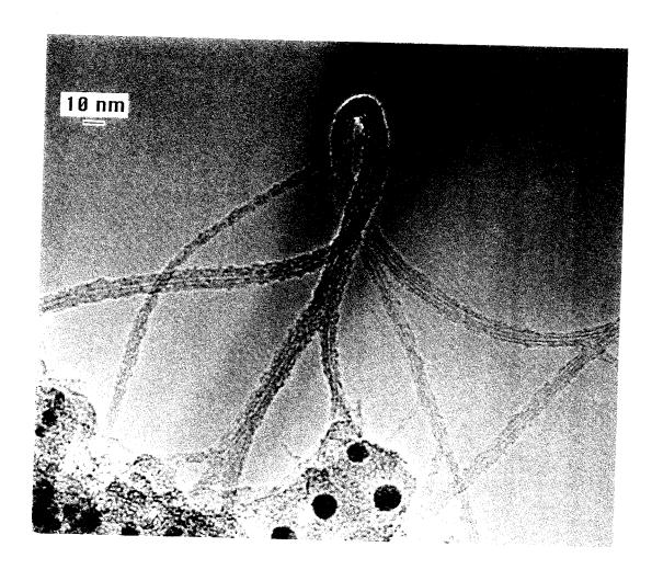
Figure 5.5: TEM image of a bundle of nanotubes with a 20 nm radius of curvature.
