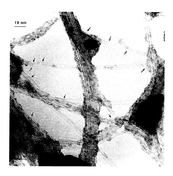
Figure 6.8: Nanotubes disintegrated under electron beam heating. The arrows point at locations where structural modification occurred due to the electron beam heating. The solid arrows are pointing to closed ends and the hollow arrows are pointing to open ends of nanotubes.
