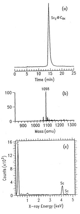
Figure 4.2: (a) HPLC trace for the  $Sc_2C_{84}$  fraction obtained using UV detection at 340 nm. (b) Mass spectrum of the  $Sc_2C_{84}$  fraction indicating > 80% purity, with roughly 10% each of  $Sc_2C_{82}$  and a species tentatively assigned to  $Sc_2C@C_{84}$ . (c) Energy dispersive spectrum (EDS) taken from a  $Sc_2C_{84}$  crystal.
