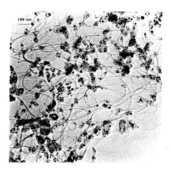
Figure 5.8: Typical low magnification TEM image of single-layer nanotubes in a soot sample made with sulfur promoter. The soot was collected on the chamber walls.
