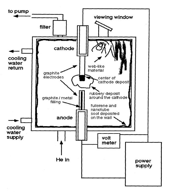
Figure 5.1: A schematic drawing of reaction chamber that was used to produce nanotubes. The soot collected from different parts of the chamber is indicated.
