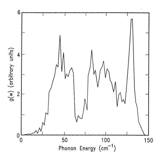
Figure 2.7: The one phonon density of states at 0K calculated for Model II.
