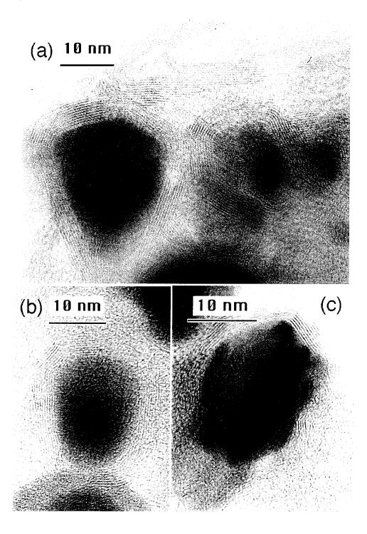
Figure 6.24: Cobalt-filled graphitic polyhedra found in soot produced with an anode containing Co and (a) S, (b) Bi, and (c) W.
