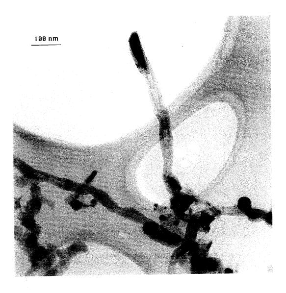
Figure 6.21: The bamboo-like carbon structures form abundantly in the rubbery deposit around the cathode when sulfur was added.
