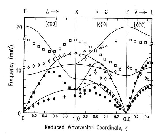
Figure 2.4: The phonon dispersion curves along  $[\zeta,0,0]$ ,  $[\zeta,\zeta,0]$ , and  $[\zeta,\zeta,\zeta]$  directions in AgBr at 4.4K (Ref. [19]). Solid curves are from Model IV and the symbols are experimental values.
