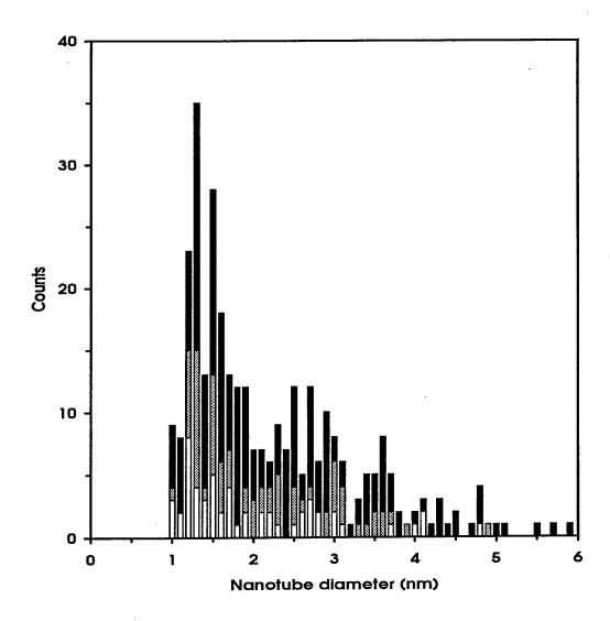
Figure 5.10: Single-layer carbon nanotube diameter distributions for samples made using 4% each S and Co powder (black bars), 4% CoS (grey bars), and 2% S from CoS and 4% Co from 1:1 ratio of Co and CoS (white bars). The uncertainty in diameter is approximately 0.1 nm for small tubes and is greater for tubes with diameters larger than 2 nm because they often exhibit radial deformation.
