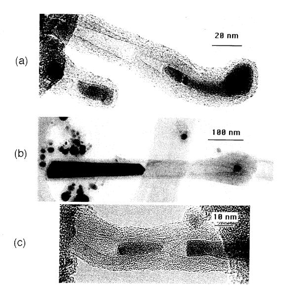
Figure 6.23: Filling of nanotubes. (a) Many of the ends of the carbon compartments contains cobalt sulfide. (b) Crystalline cobalt sulfide filled tube, with the filling more than 100 nm long. (c) Two sections in the middle of the strings of bead partially filled with cobalt sulfide.
