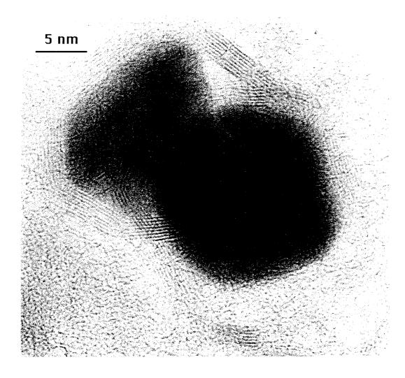
Figure 5.16: TEM image of cobalt particles encapsulated in graphitic polyhedra found in the soot away from the electrodes. The soot was produced with Co catalyst and S promoter.
