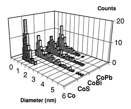
Figure 5.13: Histogram of nanotube diameter distribution of samples made from catalyst Co, Co+S, Co+Bi, and Co+Pb. The numbers of tube diameters measured were more than 150 for Co, 300 for Co+S, 150 Co+Bi, and 200 for Co+Pb. There is a 10 % uncertainty in the measured diameters.
