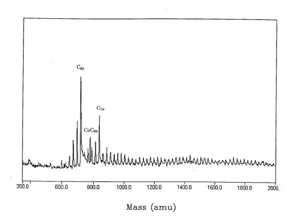
Figure 5.15: Mass spectrum of soot containing nanotubes made with cobalt catalyst.
