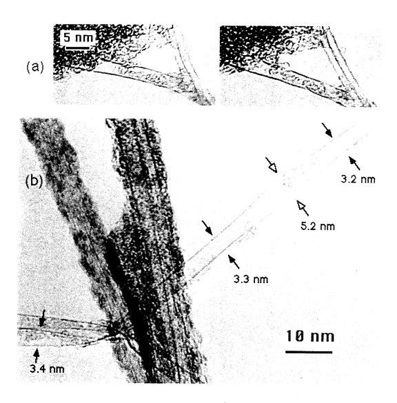
Figure 7.3: (a) A nanotube with carbonaceous material inside. The sample was rotated to verify that the amorphous material was indeed inside the tube. (b) A nanotube with material that expanded the tube wall, suggesting that the material was incorporated during the growth.
