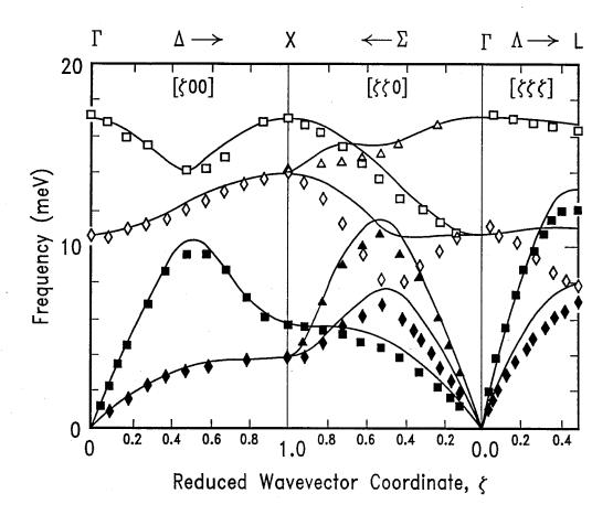
Figure 2.5: The phonon dispersion curves along  $[\zeta,0,0]$ ,  $[\zeta,\zeta,0]$ , and  $[\zeta,\zeta,\zeta]$  directions in AgBr at 4.4K (Ref. [19]). Solid curves are from Model V and the symbols are experimental values.
