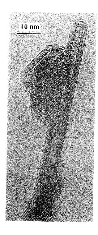
Figure 5.3: TEM of the sample from the central portion of the cathode deposit. Shown in the micrograph is a multilayer carbon nanotube and a graphitic nanopolyhedron. They form on the cathode without using a catalyst.
