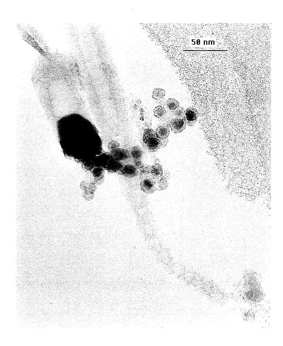
Figure 6.17: Conical graphite filament linked to a strings of carbon beads in the soot around the cathode, when Co and S were added to the anode.
