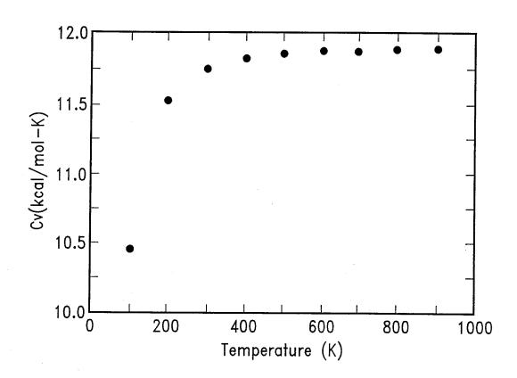
Figure 2.8: The specific heat versus temperature calculated for Model II.
