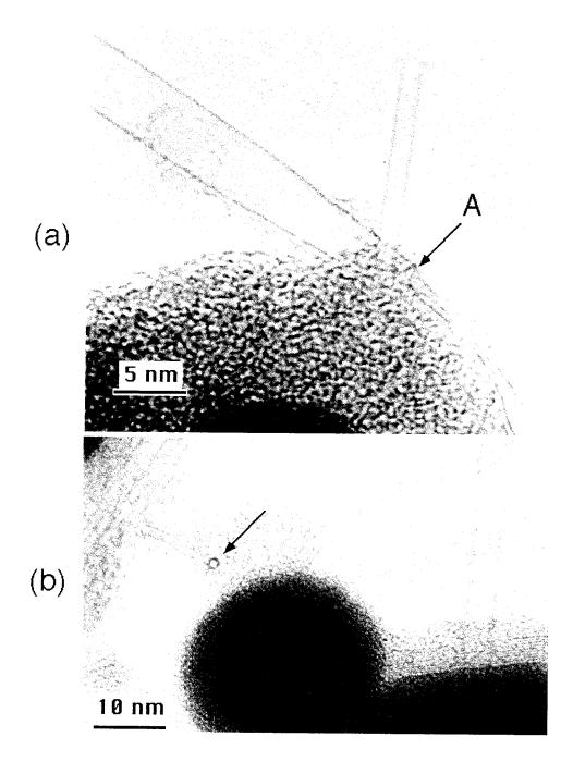
Figure 6.2: TEM of soot containing nanotubes of different diameter. (a) The larger tube is a 3.8 nm diameter tube, showing deformation near the soot. (b) The end view of a tube showing a near circular shape, indicating a cylindrical, tubular structure.
