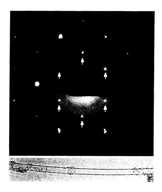
Figure 6.6: Diffraction pattern and image of a single-layer nanotube. The pattern shows the tube has a zero-helicity, armchair structure.
