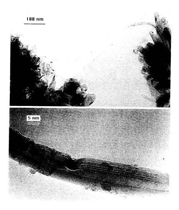
Figure 6.16: Multilayer nanotube found in the center part of cathode deposit. The anode used to generate the arc contains Co and S.
