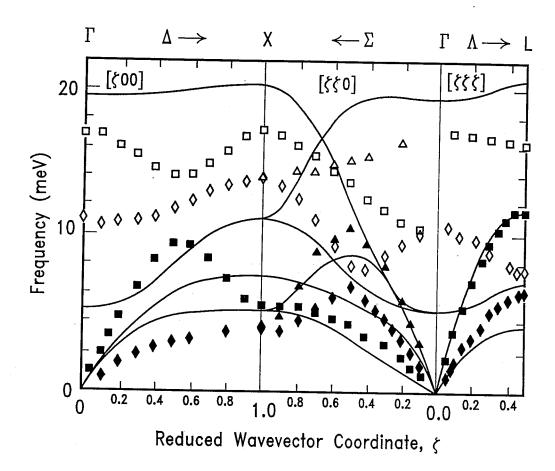
Figure 2.1: The phonon dispersion curves along  $[\zeta,0,0]$ ,  $[\zeta,\zeta,0]$ , and  $[\zeta,\zeta,\zeta]$  directions in AgBr at 4.4K (Ref. [19]). Solid curves are from Model I and the symbols are experimental values.
