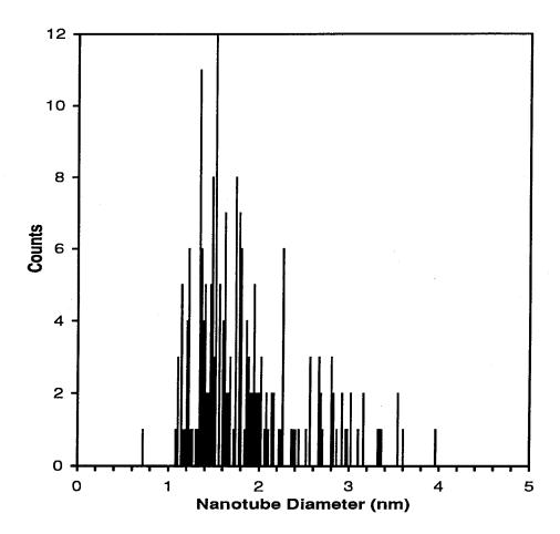
Figure 7.5: Histogram of diameter distribution of nanotubes produced with Co and Pb.
