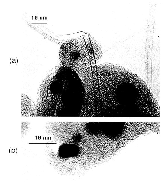
Figure 6.4: TEM showing nanotubes wrapped around the soot.
