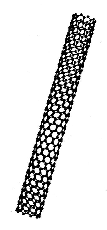
Figure 1.3: Molecular model of carbon nanotubes. The honeycomb structure of nanotubes was confirmed by transmission electron microscopy studies.
