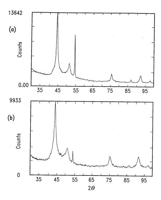
Figure 5.14: X-Ray powder diffraction spectra of (a) soot made with Co and (b) soot made with Co and S. The peak at  $2\theta = 45$ ° is due to graphitic carbon structure. In both spectra, only the fcc phase of Co was detected.
