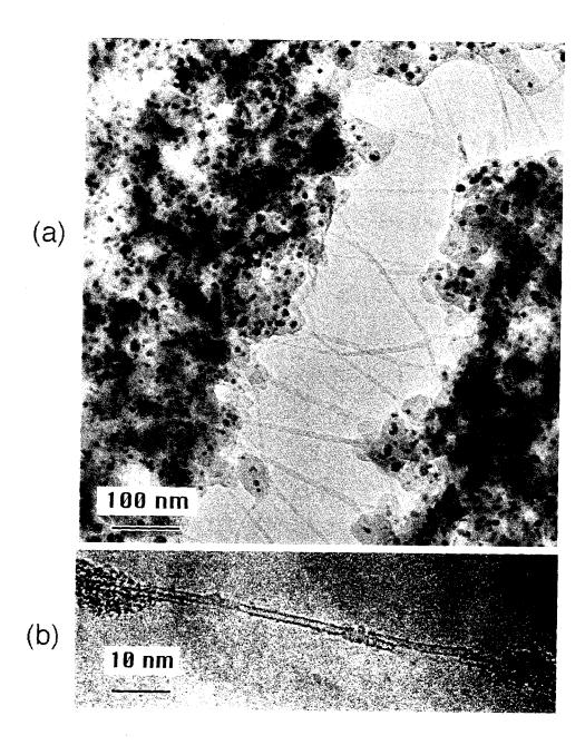
Figure 5.2: (a) Transmission electron micrograph (TEM) of web-like material showing strands of thread-like fibers and cobalt clusters (dark spots) embedded in carbon soot particles. (b) TEM of bare sections of single-layer nanotubes.
