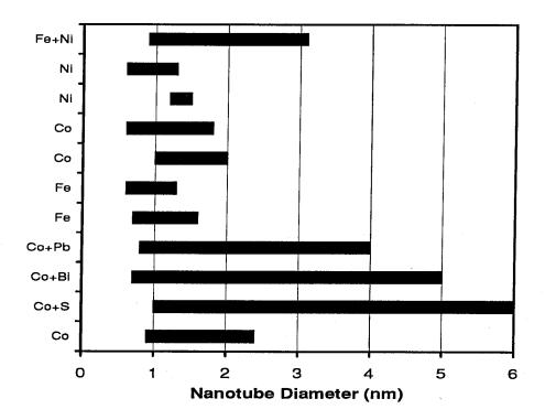
Figure 7.1: Ranges of nanotube diameters produced by using different catalyst and promoters.
