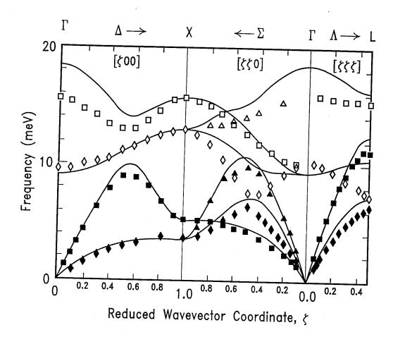
Figure 2.3: The phonon dispersion curves along  $[\zeta,0,0]$ ,  $[\zeta,\zeta,0]$ , and  $[\zeta,\zeta,\zeta]$  directions in AgBr at 4.4K (Ref. [19]). Solid curves are from Model III and the symbols are experimental values.
