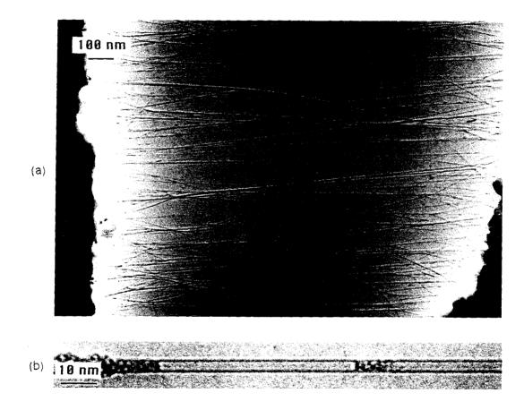
Figure 5.6: (a) TEM of nanotube bridges over a split in the soot deposit. (b) High resolution TEM image of a nanotube containing some amorphous material.
