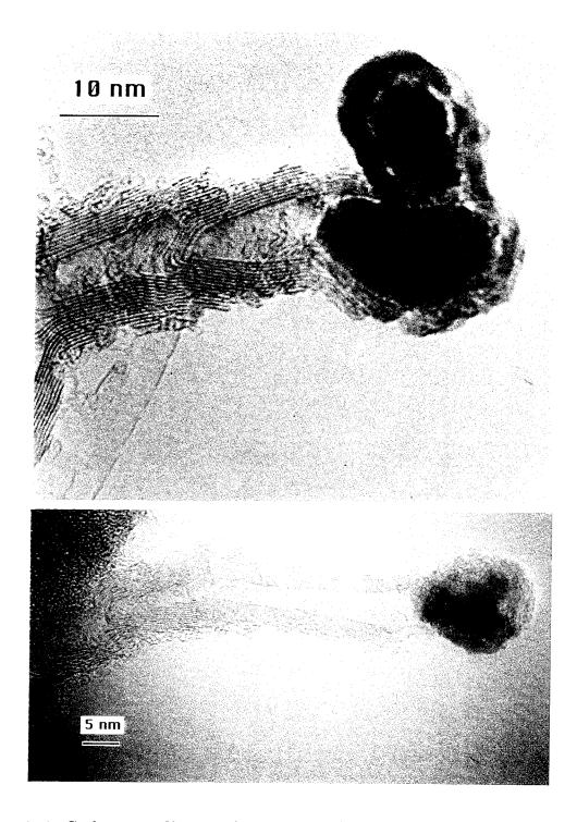
Figure 6.19: Carbon nanofibers in the soot around the cathode, when Co and S were added to the anode. The particles at the end of the fibers are cobalt sulfide crystals.
