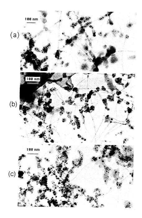
Figure 5.4: TEM image of the soot produced using various concentrations of Co in atomic percentage of (a) 2%, (b) 4%, and (c) 6%. The highest yield under these conditions described in the text is for 4% Co. The threads apparent are individual or bundles of nanotubes. Most of the nanotubes are covered with carbon soot.
