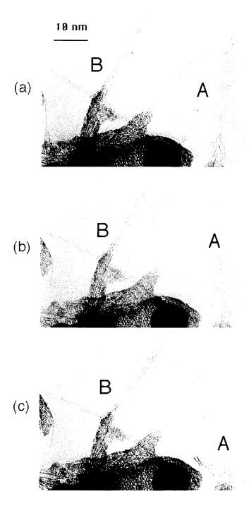
Figure 6.11: Nanotube bundling imaged in real time. (a) A tube bridge between bundle A and B. (b) Bundle A disintegrated, and the tube is pulled towards bundle B. (c) The tube eventually bundled with B.
