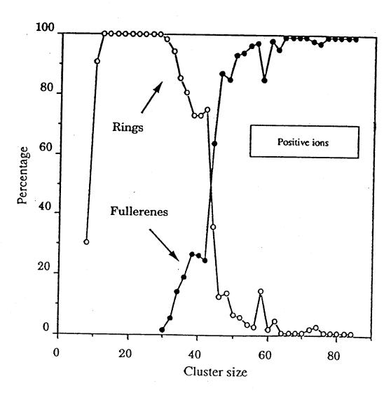
Figure 7.4: Plots of percentage of planar carbon rings and fullerenes as a function of carbon cluster size (from Ref. [35]).
