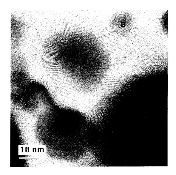
Figure 5.17: Co crystallites encapsulated in graphitic polyhedra, produced with Co and Bi. The crystallite marked A is a 20 nm diameter fcc-Co crystallite encapsulated in 17 layers of graphene sheets, which have a constant spacing comparable to that of bulk graphite. The particles marked B, C, and D are also fcc-Co crystallites, similar to those produce without Bi, and the particle marked E is a pure Bi particle.
