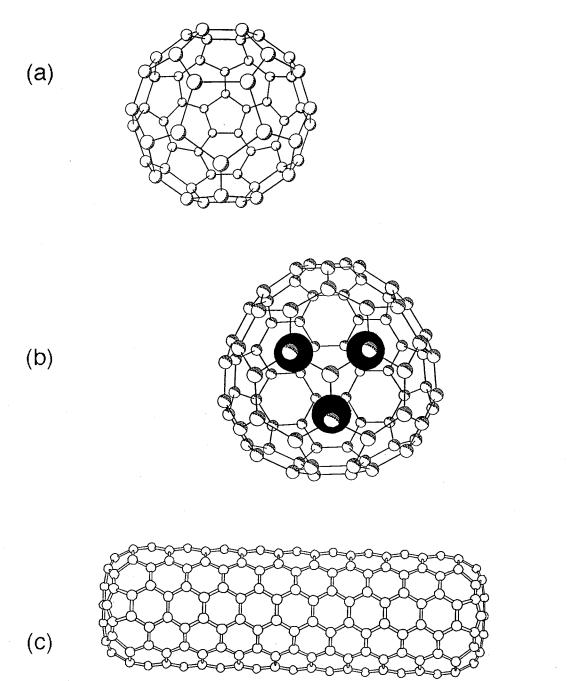
Figure 1.1: Various carbon structures formed by self-assembly: (a) Fullerene  $C_{60}$ , (b) Endohedral Metallofullerene  $Sc_3@C_{82}$ , and (c) carbon nanotube with an armchair structure (from Ref. [19]).
