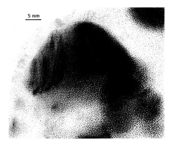
Figure 5.18: Co crystallites encapsulated in a graphitic polyhedron, produced with Co and W. There are two crystallites encased in the nanopolyhedron.
