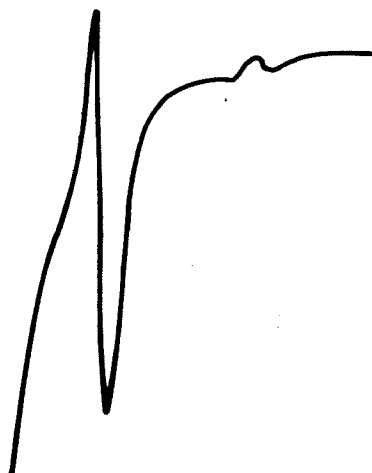
Figure 17 Auger spectra of two Ni-covered Si (111) samples. At the higher deposition temperature, the Si L 23 V signal (92eV) shows a higher intensity; it denotes the Si is closer to the Ni surface.
