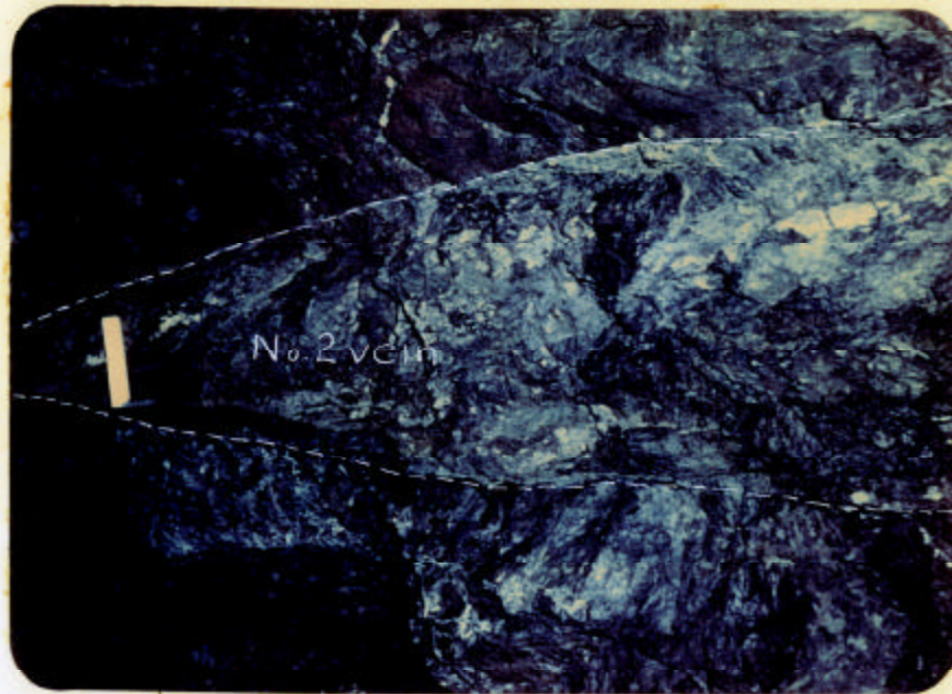
No. 2 vein, 250 level east, drift back. Note narrowing of vein to left within more competent body of feldspar porphyry. The vein widens to three feet, 20 feet to the right of the location photographed, where it enters Mine series tuffs. The scale shown is six inches long.
