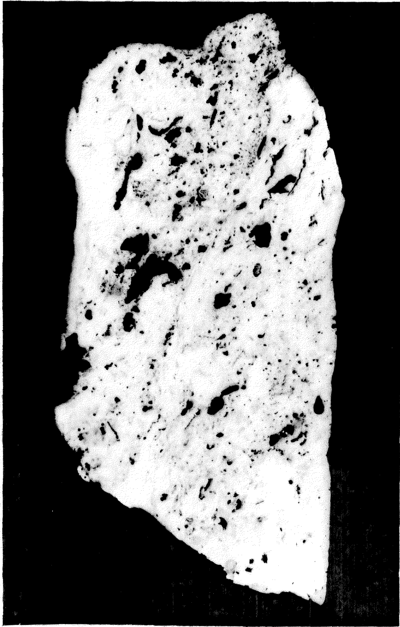
Autoradiograph of "diffuse" pitchblende (black) comminuted and replaced in chloritic quartz (white). No. 5 vein, 54 ore shoot. xl
