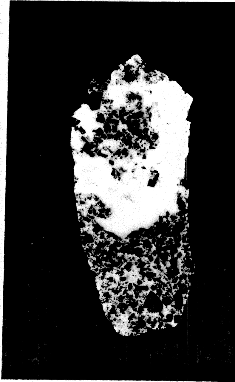
Autoradiograph of brecciated pitchblende (black) in chloritic, chalcopyrite "ore" quartz gangue (white). No. 2 vein, 21 ore shoot. xl
