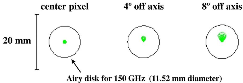
(b) Geometric spot diagrams. The optical performance of the lenses is completely diffraction-limited, as the above comparisons between the 150 GHz Airy disk and geometric spot diagrams for various focal plane locations show.
