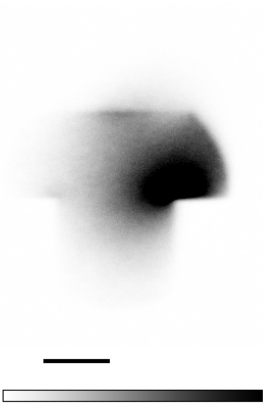
Figure 4.3. Linear histogram image of the x-y location of a bead in the “T” potential. The black bar represents 50 nm. The intensity scale here goes from light representing 0 times the particle was found at that location to dark representing 3976, meaning the particle was found in that x-y location bin 3976 times.
