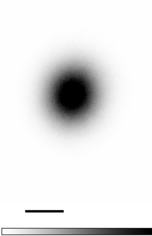
Figure 4.6. Linear position histogram for bead in trap with laser set at maximum power for autocorrelation measurements. Black bar represents 50 nm distance. Intensity scale goes from 0 to 1402.
