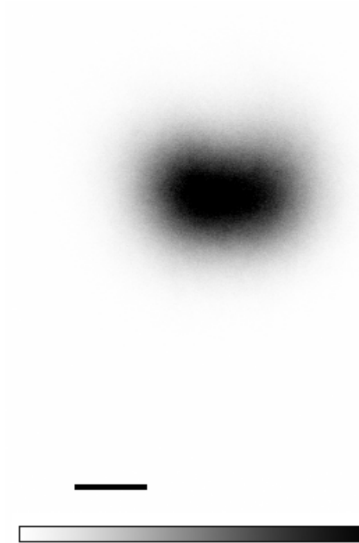
Figure 4.17. Linear position histogram for the autocorrelation data taken to calibrate the trap for the “Pacman” potential. Black bar represents 36 nm distance. Intensity scale goes from 0 to 962.
