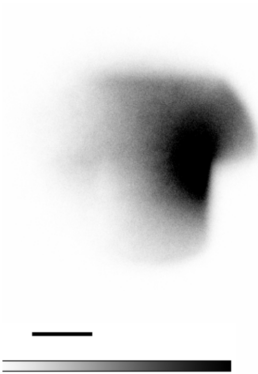
Figure 4.21. Linear histogram image of the data taken for the first attempt to produce the “T” potential. The black bar represents 50 nm. The intensity scale goes from zero to 1003.
