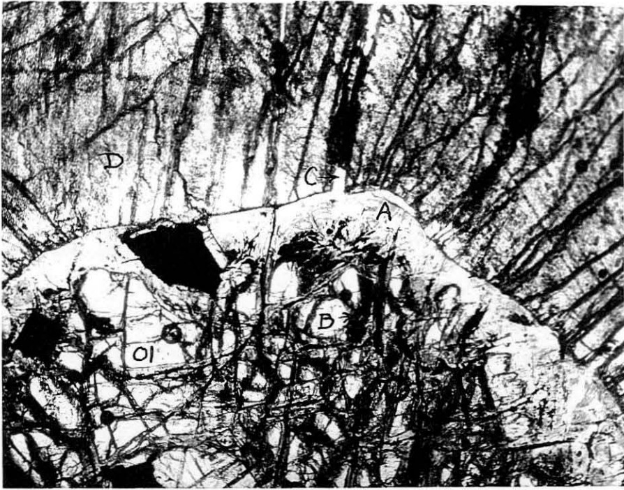
Figure 30. Photomicrograph of a thin section of partially serpentinized peridotite (x30). A subhedral crystal of olivine (Ol) has been partly altered to antigorite (A) and bowlingite (B). Diopside (D) containing much very fine-grained magnetite is interstitial to the olivine. Fractures filled with chrysotile (C) occur radially distributed in the diopside around the olivine crystal. Black areas are magnetite.
