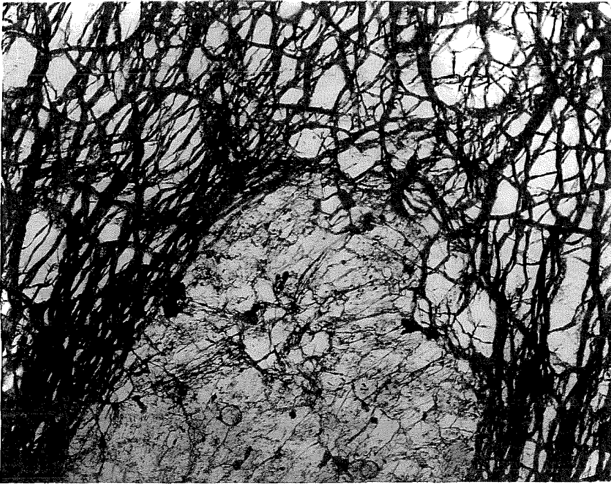
Figure 26. Photomicrograph of a thin section cut from a small dunite sill in olivine-pyroxenite (x30). The fractured, but undisturbed, subhedral olivine grains enclose an aggregate of anhedral diopside grains. The black, opaque mineral associated with the diopside is magnetite. The olivine grains are approximately 1 mm in size. The fractures, which curve around the inclusion of diopside grains, contain bowlingite.
